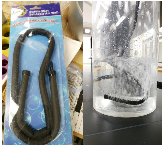
Figure 3-2: Example of air diffusion in clean water with Bubble Mist – Bendable Air Wall
