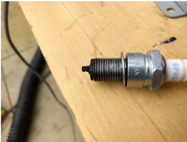
(a) Spark plug with carbon build-up on the tip (b) Engine valves showing no damage but large amount of carbon deposits
