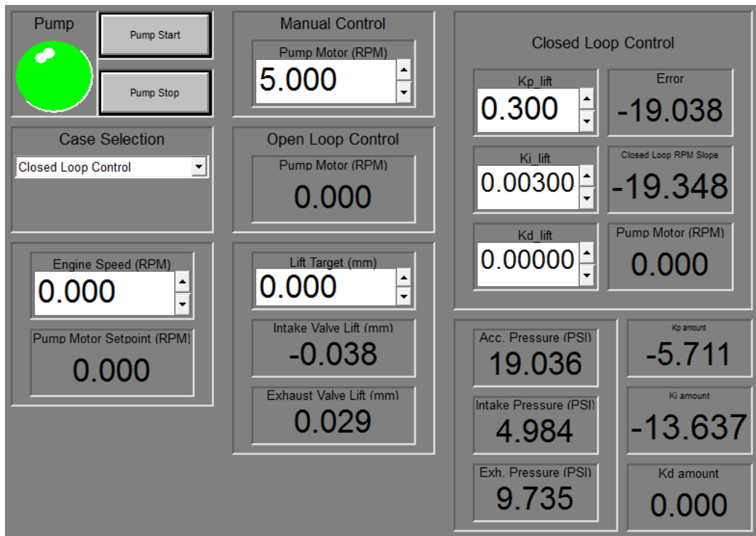
Figure 4.18: User interface for selecting manual, open loop, or close loop PID control to reach a desired valve lift for an engine speed
