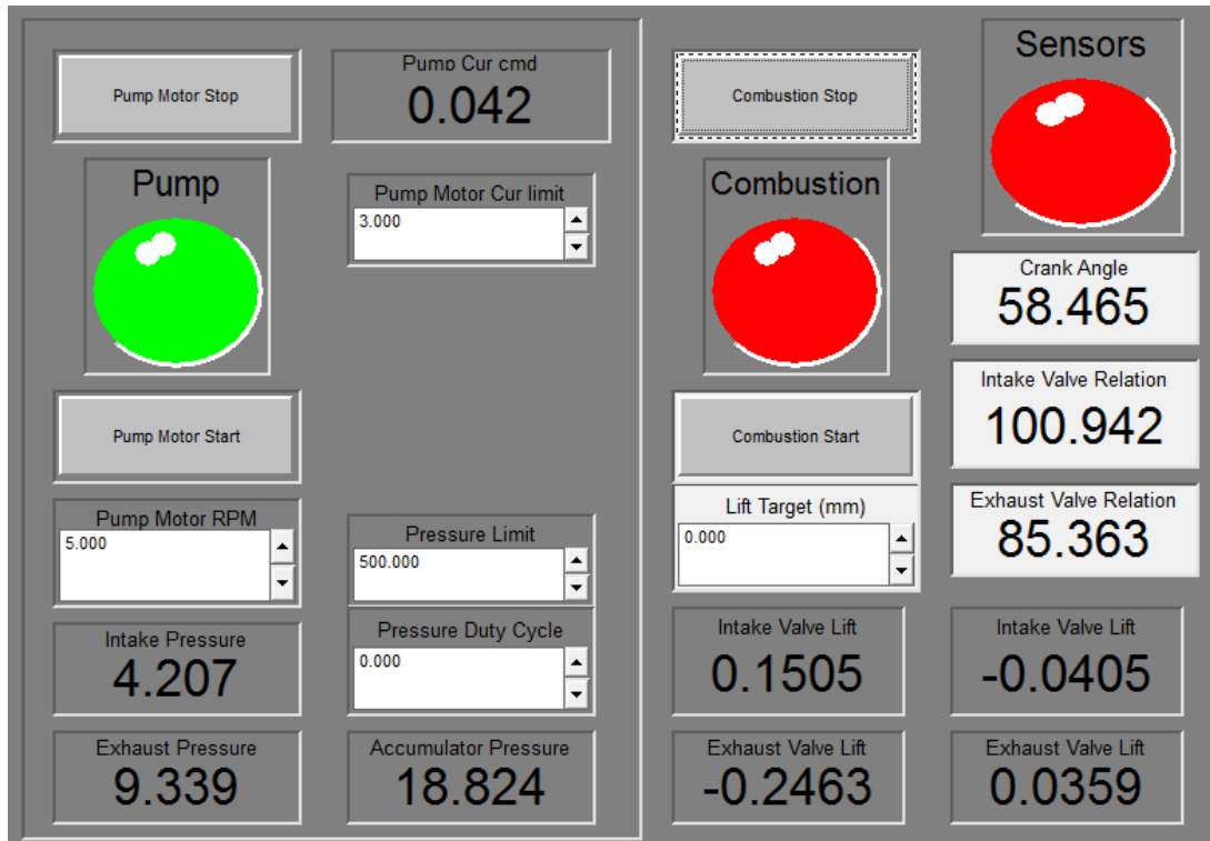
Figure 4.16: Control Desk user input interface allowing manual control of pump, lift target, combustion start and read outs of pressures and valve lifts
