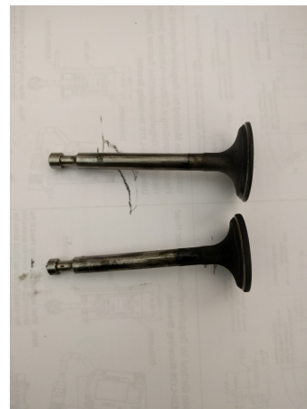
(a) Spark plug with carbon build-up on the tip (b) Engine valves showing no damage but large amount of carbon deposits
