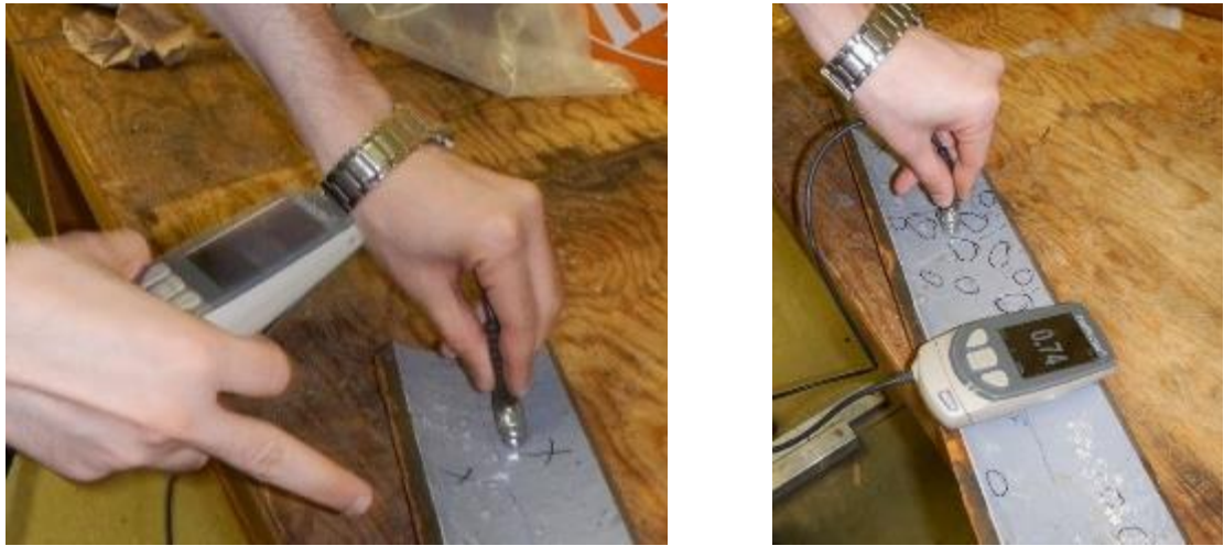
Figure 2.9: Thickness measurements using a Positector 6000 device.
