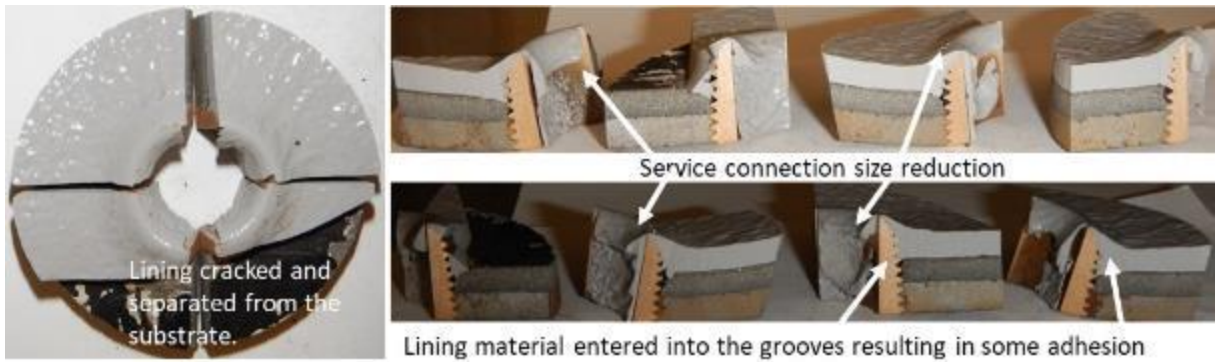
Figure 3.18: Service connection 2B6-2 for Rack bore cleaned section.
