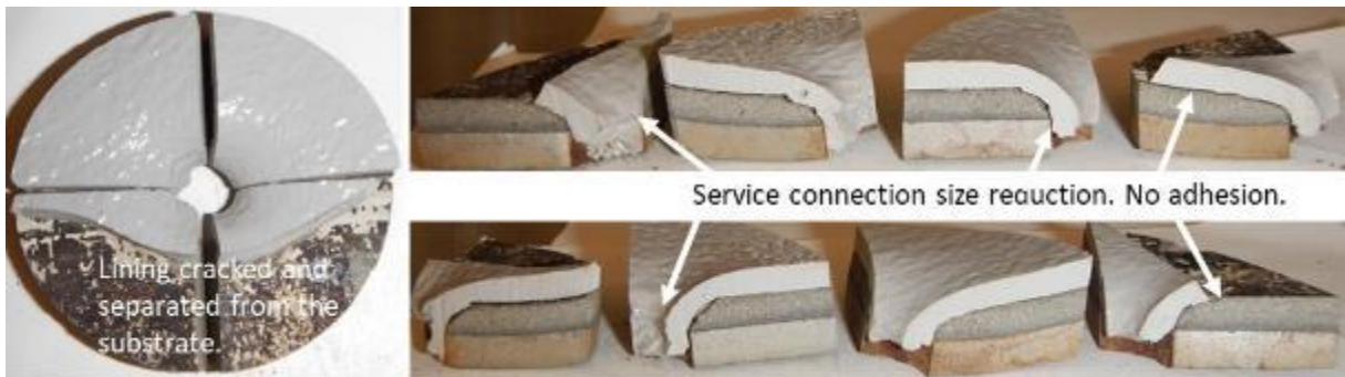
Figure 3.17: Service saddle 2B4 for Rack bore cleaned section.
