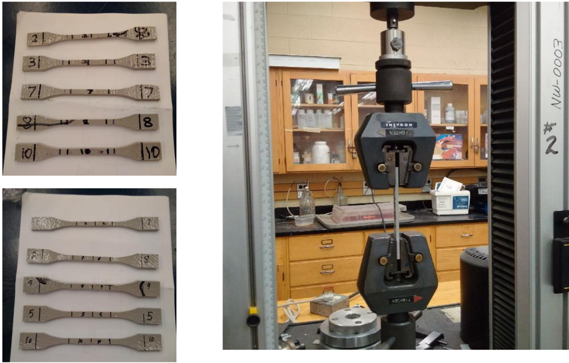
Figure 3.30: Specimens and tensile test setup.
