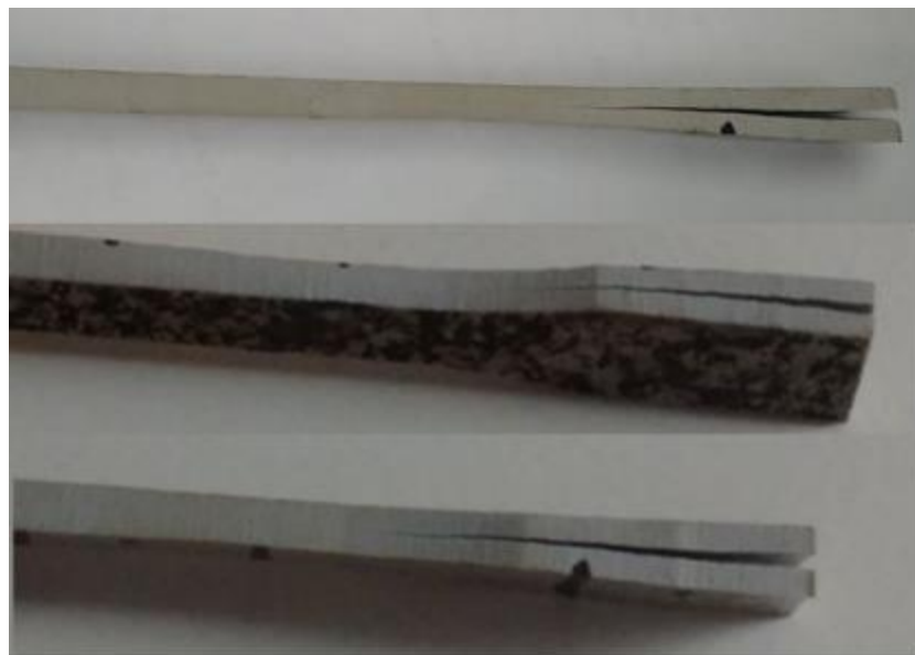
Figure 3.29: Separation of two lining layers in some tensile samples.
