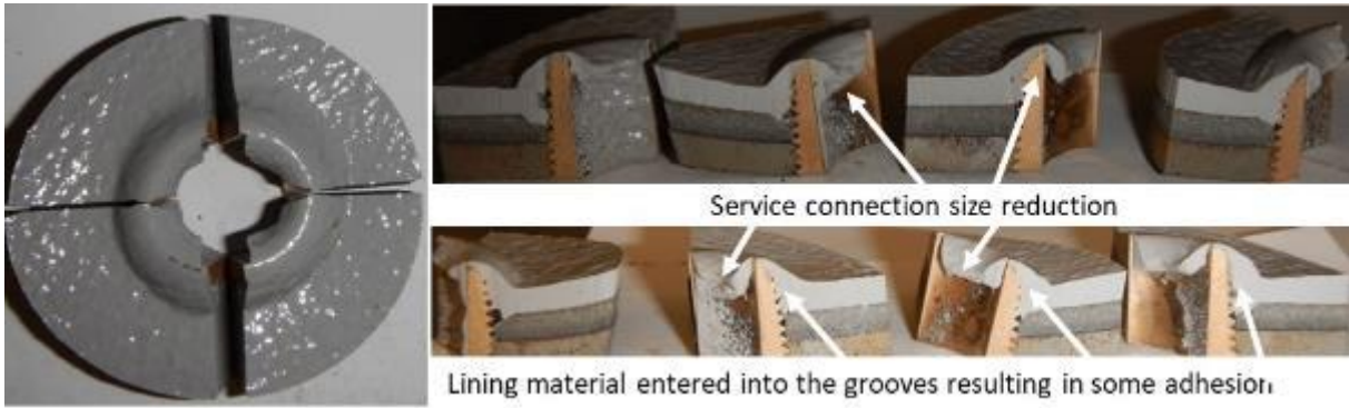
Figure 3.19: Service connection 2B4 for Rack bore cleaned section.
