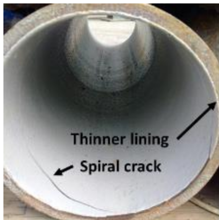
Figure 3.11: Lining thickness variation at two ends of the same pipe section with spiral crack visible in the thinner lining.
