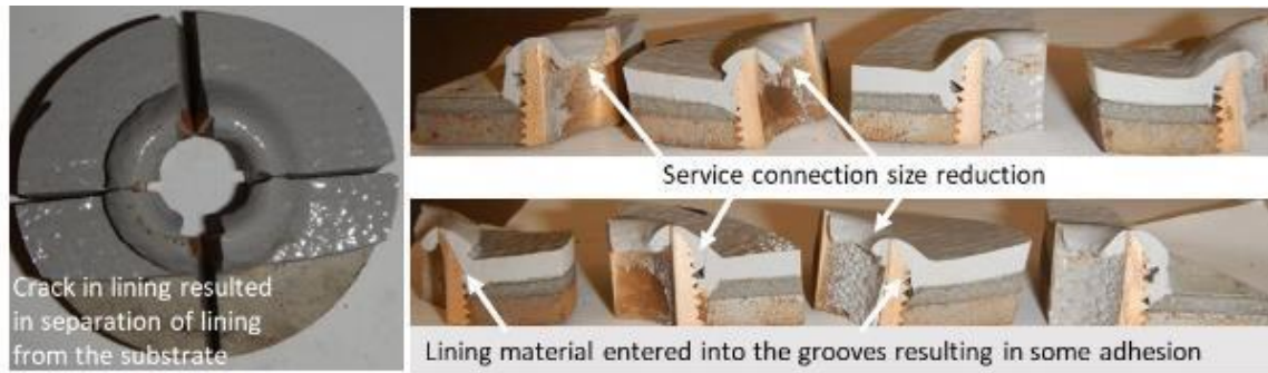
Figure 3.22: Service connection 3B6-2 for Water jet cleaned section.
