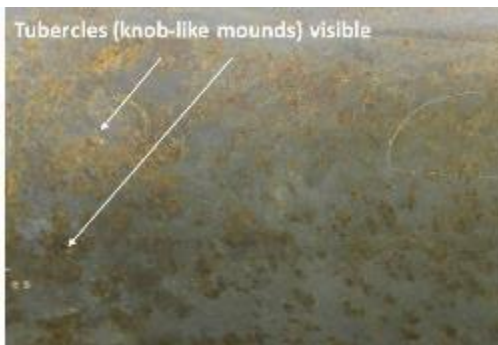
(b) Section 2 cleaned using ID-TEC SR-Series high pressure water jet tool.
