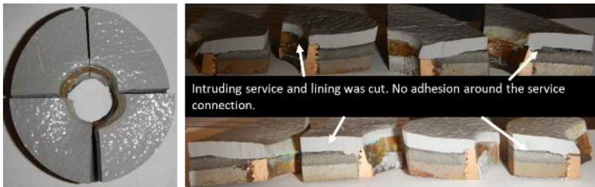
Figure 3.15: Service connection 1B3-1(1) for Tomahawk cleaned section.
