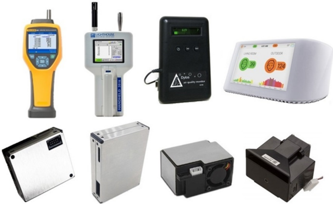
Figure 3.1: Photograph of the evaluated sensors. Clockwise from top left: Fluke 985, Handheld 3016, DC1100 Pro, Node, DN7C3CA006, SDS 021, PMS 7003, and PMS A003.
