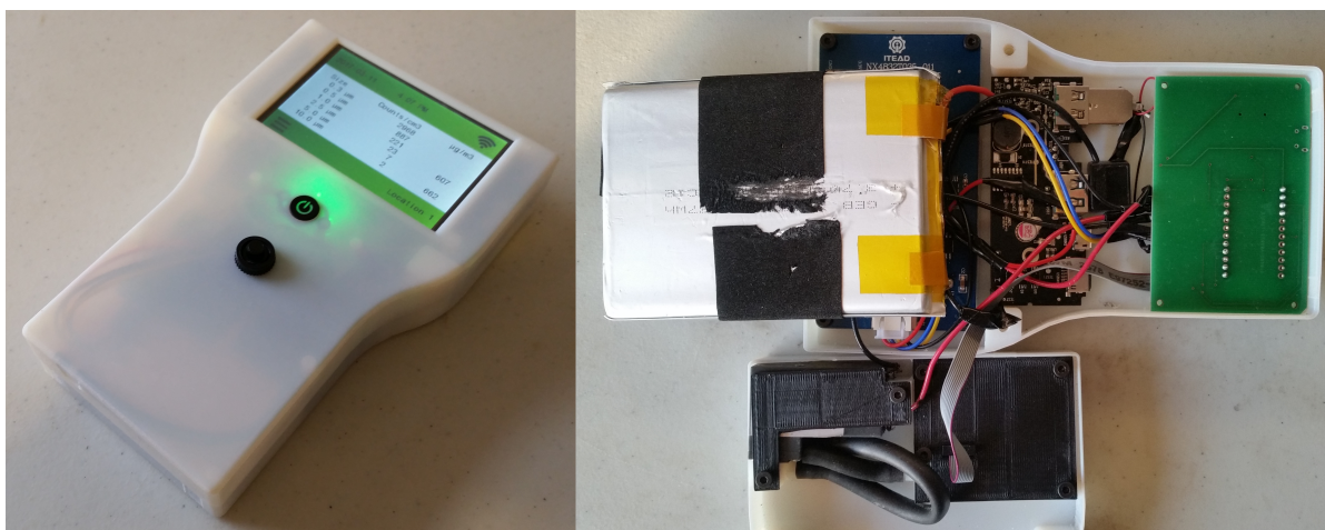
Figure C.2: Photograph of the first design iteration (left) and internal components (right).
