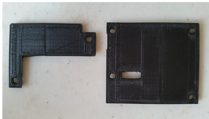
Figure C.4: Parts 3D printed to secure the pump (left) and PMS A003 (right) in the casing.
