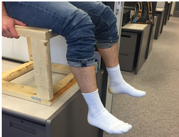
Figure 3.9: Seated pose used to capture a complete foot scan using Kinect Fusion.
