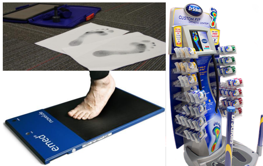
Figure 2.2: Examples of pedograph systems. Top-Left: The ink pedograph [57], Bottom-Left: The emed@electronic pedograph system [60], Right: The Dr. Scholls Custom Fit Orthotics Center [37].
