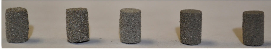
Figure 3.3: Qualitative comparison between the build quality of the different sample types made from powder types (from left to right) A, B, C, D and E
