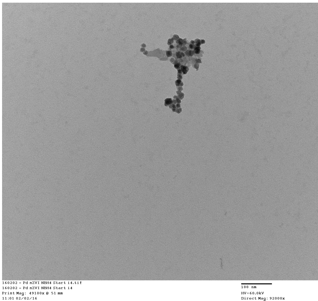
Figure B.4 Image of a sample of synthesized Pd nZVI prior to use in batch experiments taken using transmission electron microscopy (TEM). High voltage was set at 60 kV. The direct magnification factor is 92,000.
