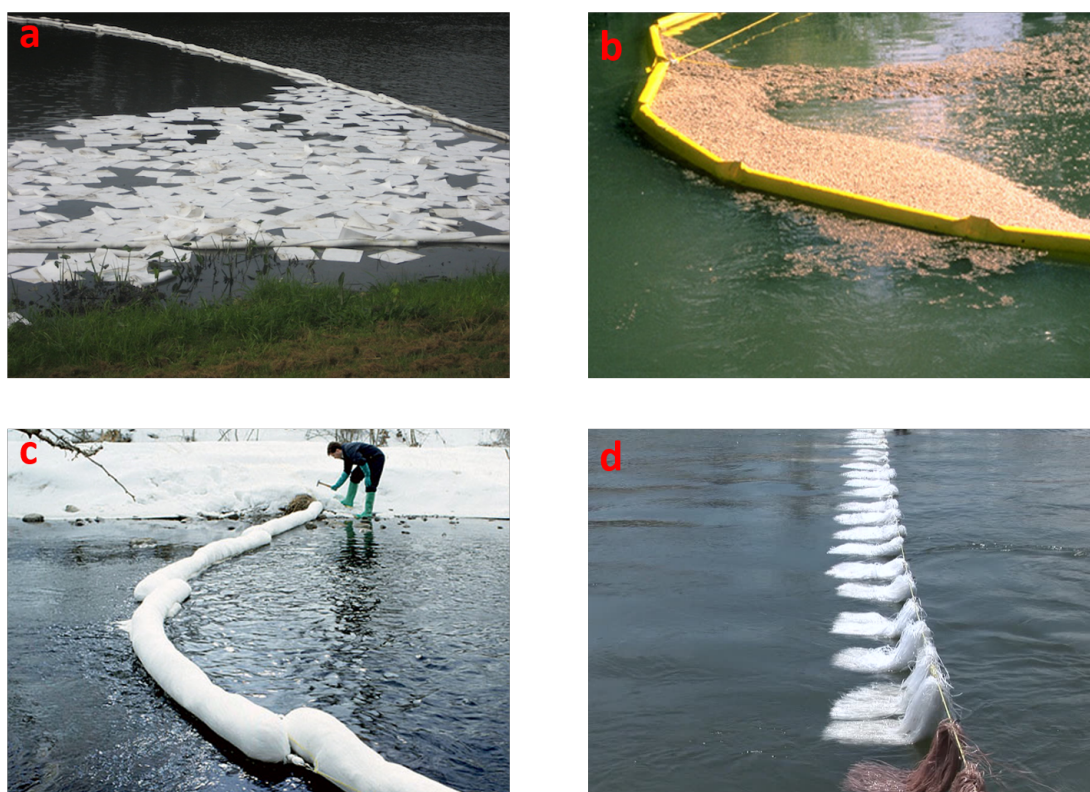
Figure 2.1: 4 types of sorbents; a)Type 1 (sheets), b)Type 2 (loose) , c) Type 3 (booms) and d)Type 4 (pom-poms)
