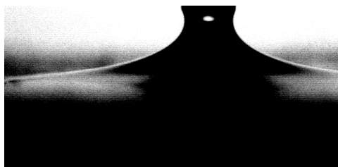
Figure 4.6: Kerosene oil being detached from the tip of the needle
