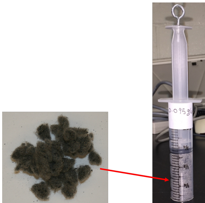
Figure 3.5: Left: Short fibers; Right: Sample holder for porous media
