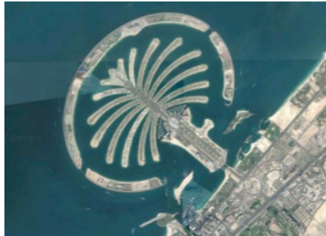
FIGURE 23 The Palms Jumeirah development is very unconventional as it begins eroding the second the fill hits the water; calling to question the long term effects on the surrounding environmental systems of beach erosion and deposition.
