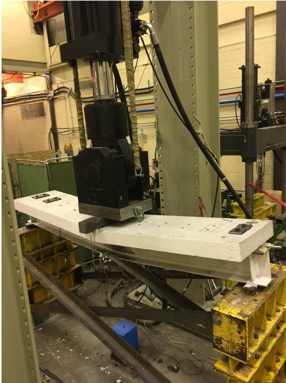
Figure 4–35: Ultimate strength testing frame and setup of Specimen B3
