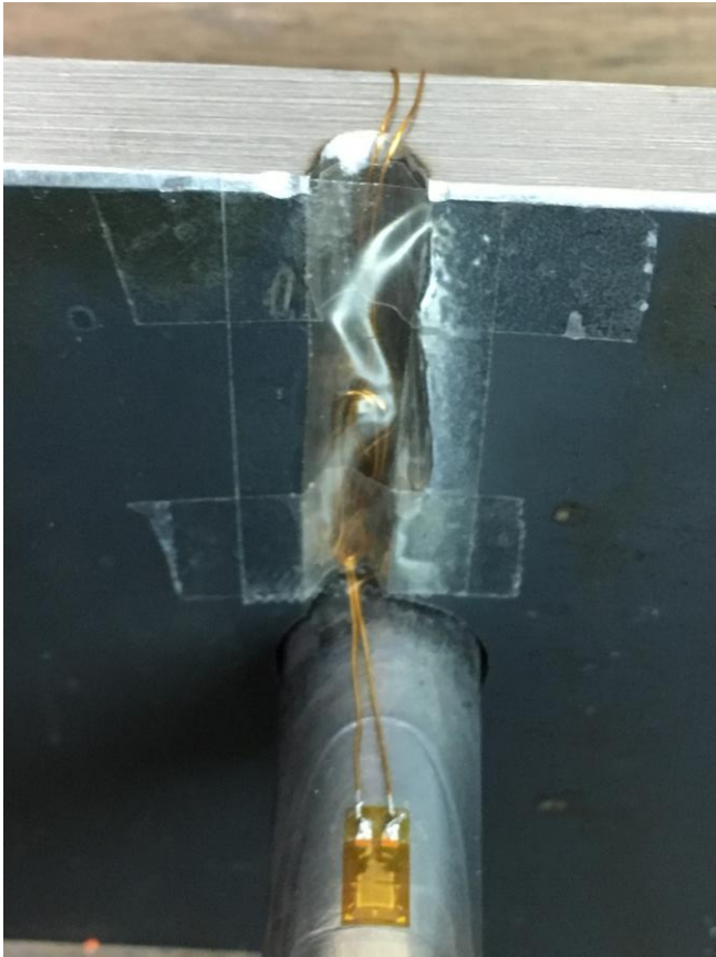
Figure 3-7: Strain gauge wiring
