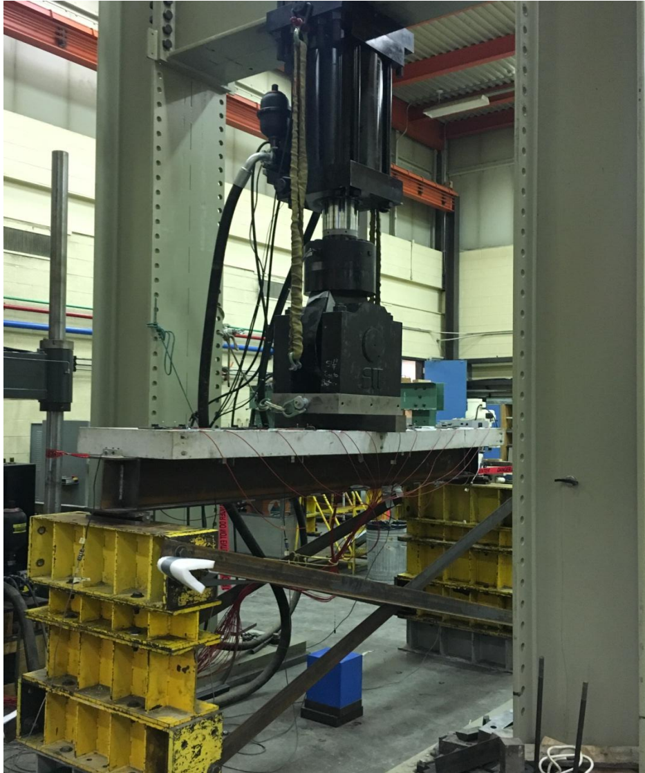
Figure 3–15: Ultimate strength testing frame and setup
