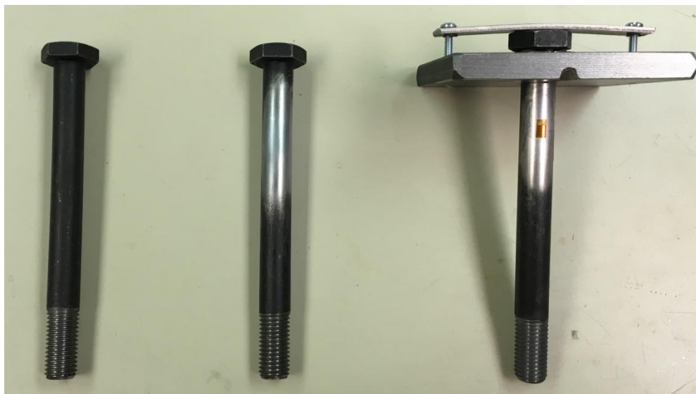
Figure 3–6: Through-bolt strain gauge preparation
