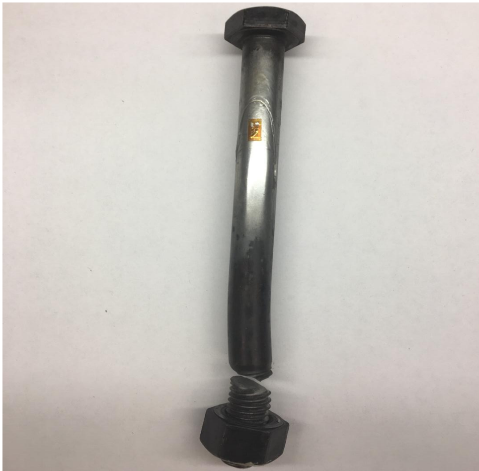
Figure 4–36: Typical through-bolt failure
