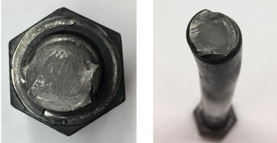
Figure 4–37: Typical failure shear surfaces of hex nut (Left) and through-bolt (Right)
