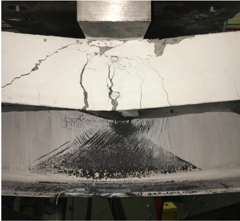
Figure 4–34: Whitewash cracking at the midspan of Specimen B3 at failure
