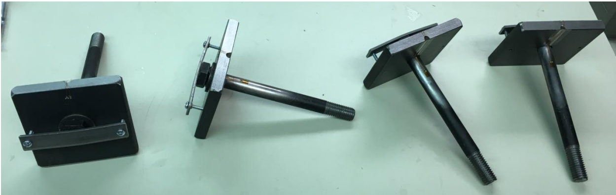
Figure 3-8: Fully instrumented through-bolts
