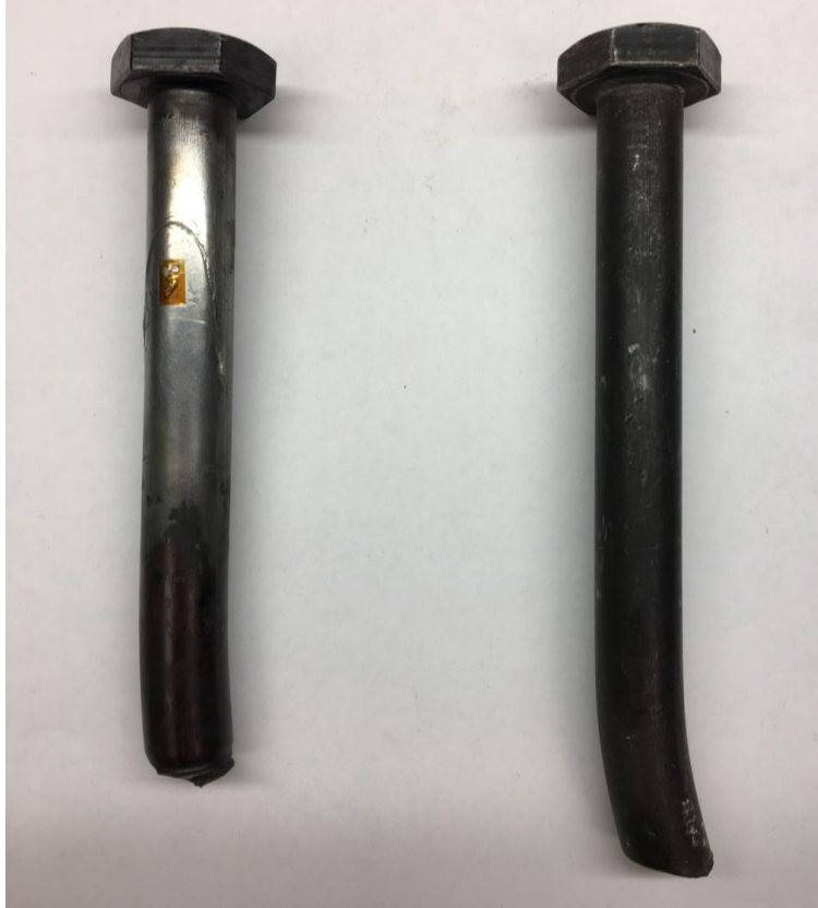
Figure 4-47: Comparison of through-bolt failures from beam test (Left) and push test (Right)
