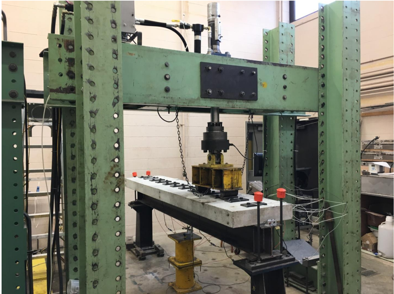
Figure 3–14: Laboratory testing frame and setup for stiffness and fatigue tests
