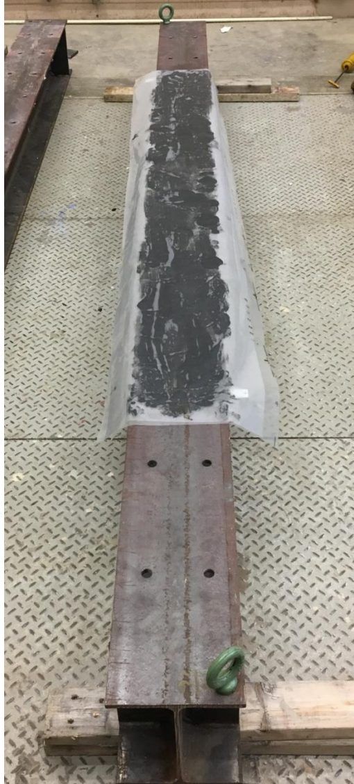
Figure 3–13: High pressure grease placed between polyethylene sheets
