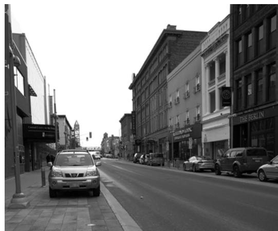
Fig. 168. King Street in Downtown Kitchener in front of the Berlin. The transition between the road and curb is minimized by using a curb similar to one of a driveway entry.
