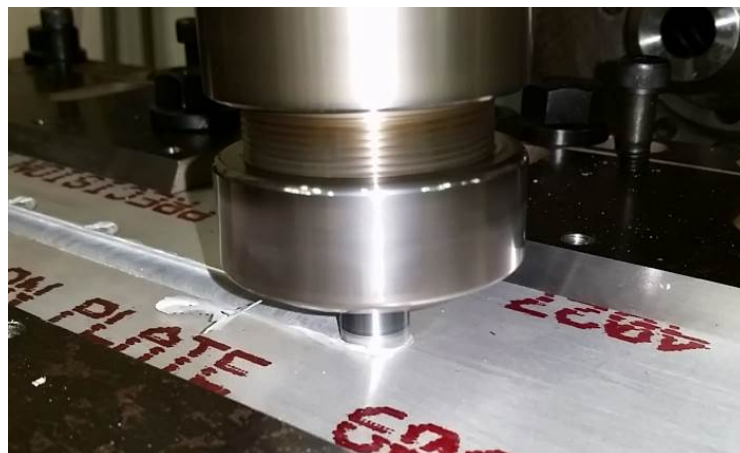
Figure 1.1 Friction stir welding process
