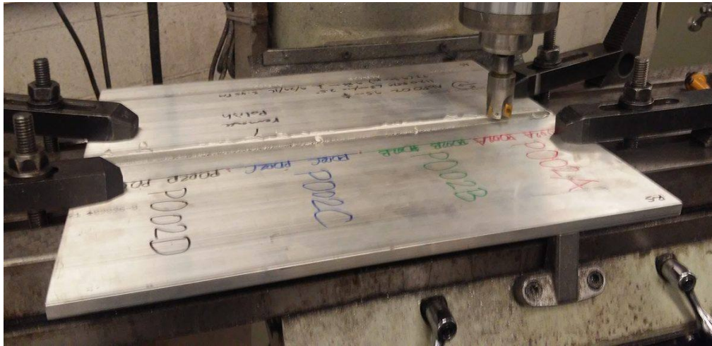
Figure 3.7 Milling of the toe flash for polished condition
