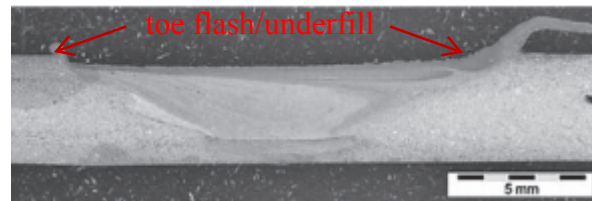
Figure 2.8 Macrograph of FSW joint with toe flash (Podržaj, Jerman, & Klobčar, 2015)
