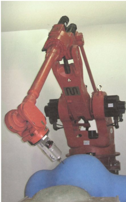
Fig. 71 - Robotic Arm Cutting Blobwall Brick Greg Lynn FORM
