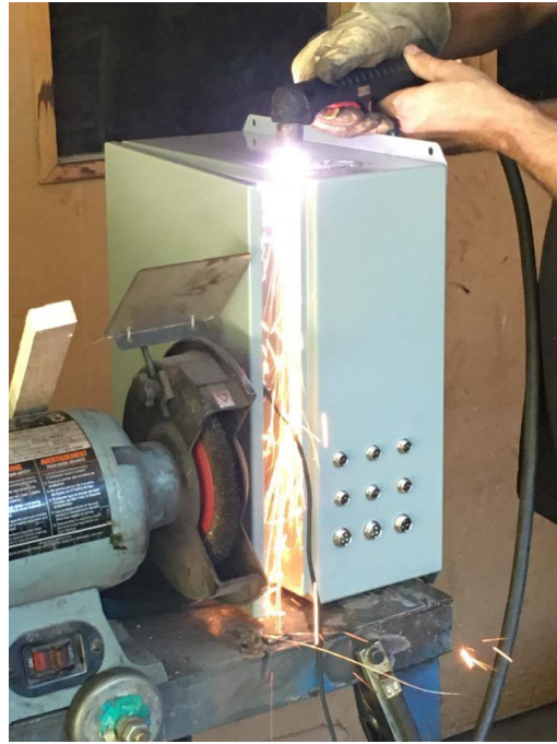
Fig. 155- Plasma-Cutting of Interface Ports in Case
