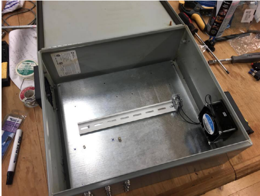
Fig. 154- DIN Rail System in Hammond Case
