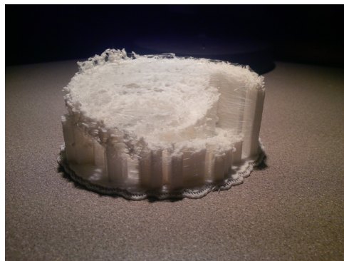
Fig. 88 - Supporting Material Removal Frustration
