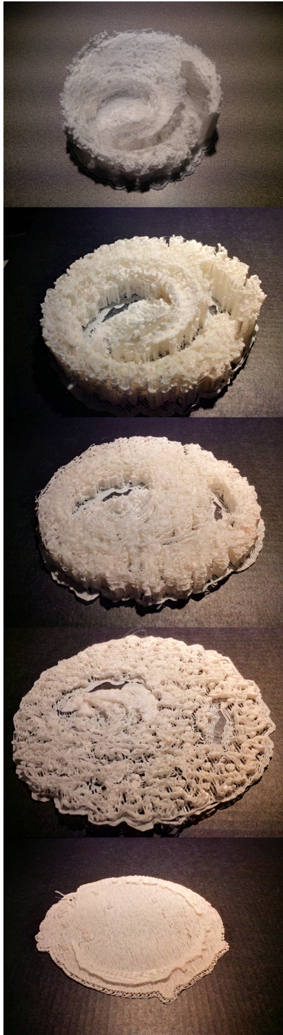
Fig. 87 - Snapshot Print Failures
