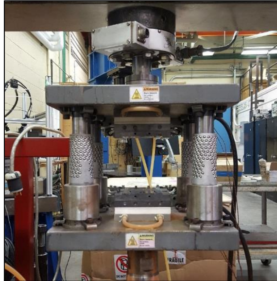
Figure 22: Custom tooling assembly on the Instron frame
