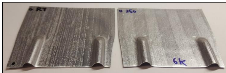
Figure 75: O-temper PF without lubrication at 25°C (left) and 250°C (right)
