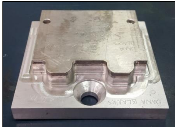
Figure 105: Blank machining jig for TC4
