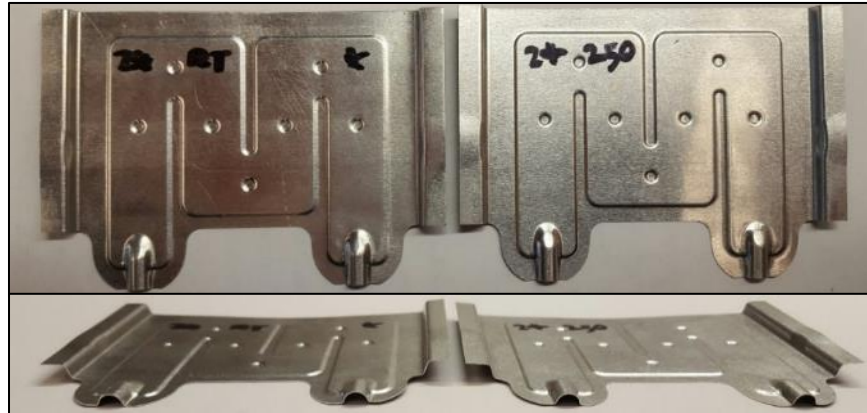
Figure 108: SHC formed with H24-temper sheet at 25°C (left) and 250°C (right) using TC4
