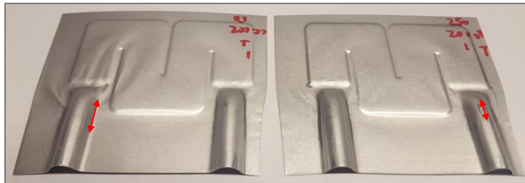
Figure 91: TC3 PF geometry formed with H24-temper sheet at 25°C (left) and 250°C (right) with Teflon lubrication
