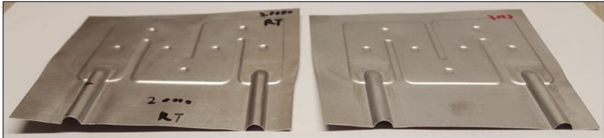
Figure 96: TC3 PF formed with full punch load (left) and reduced punch load (right) at 25°C then formed to FF at 25°C
