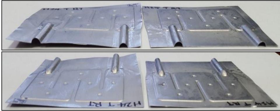
Figure 98: PF formed at 25°C then formed to FF at 25°C (left) and 250°C (right) using TC3
