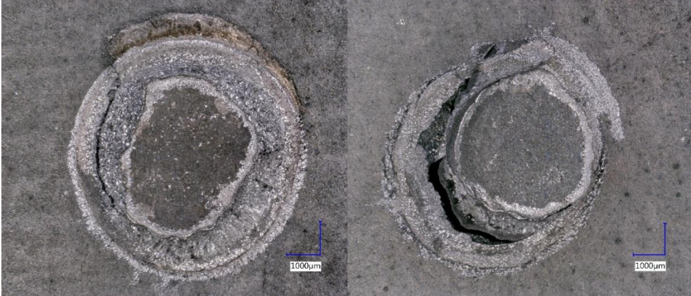
Figure 73: Cross tension single (left) and double (right) fracture images
