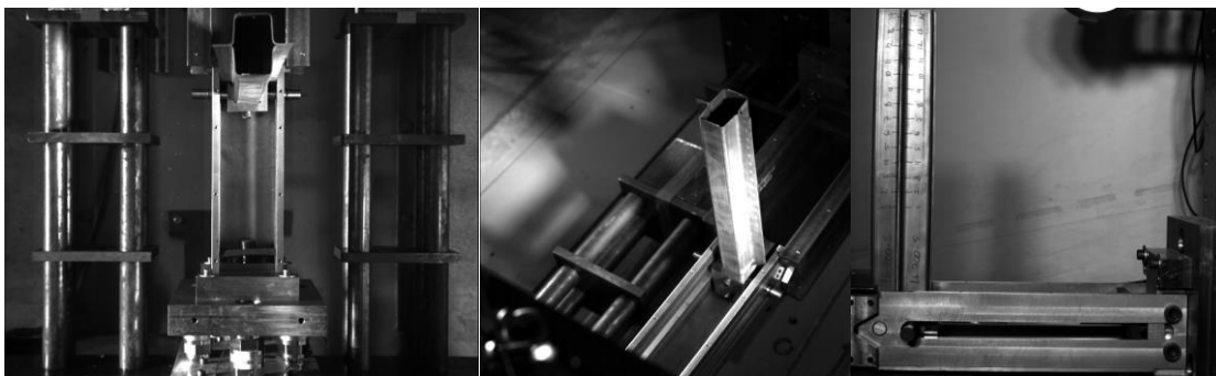
Figure 71: Still images of Mode I dynamic set up from top (left), isometric (center), and side (right) views
