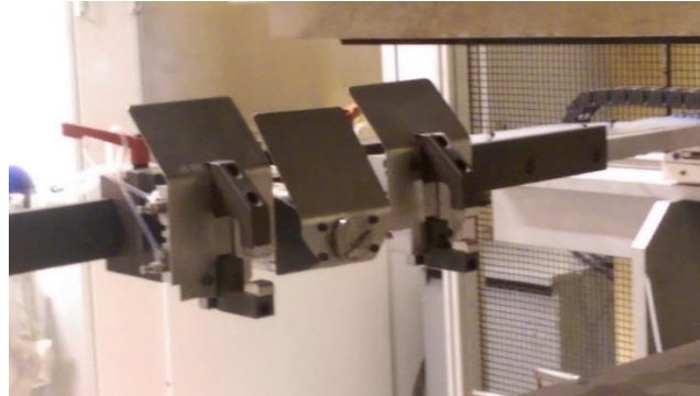
Figure 38: Gripper incorporated within the blank transfer system
