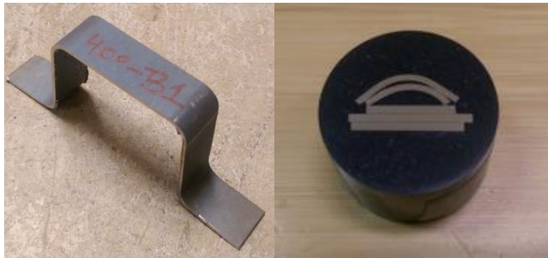
Figure 51: Hat channel hardness strip (left) and mounted specimen (right)
