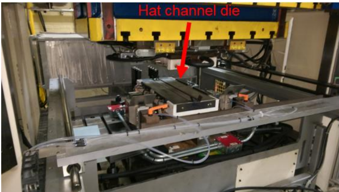
Figure 48: Hat channel tool set installed in Macrodyne press
