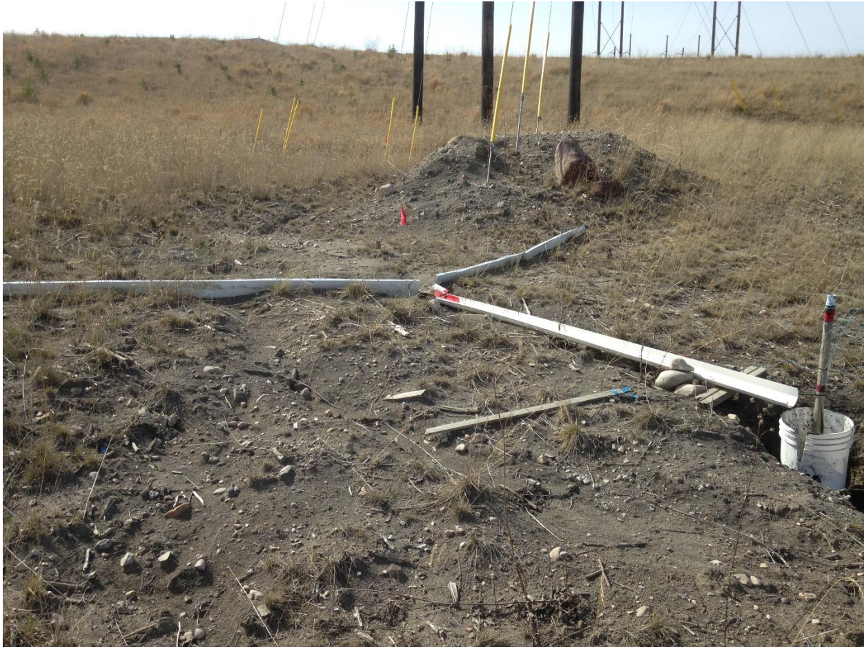
Figure 3-4. Flume open to the southeast hillslope used to estimate runoff depth and collect DOC samples. Bucket contains a well with a Schlumberger Mini- Diver pressure transducer.
