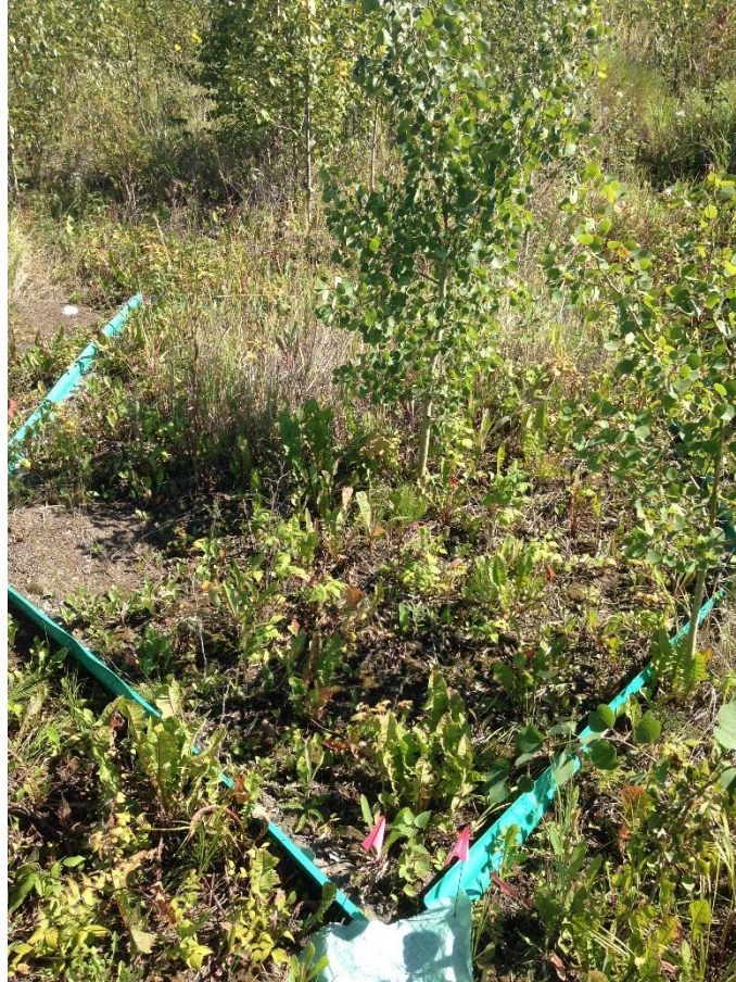
Figure 3-3. An enclosed runoff collector, located on the east slope, used to collect DOC samples and estimate runoff depth in 2016. Vegetation cover was extensive, and tree height within this photo was ~1.5 m.
