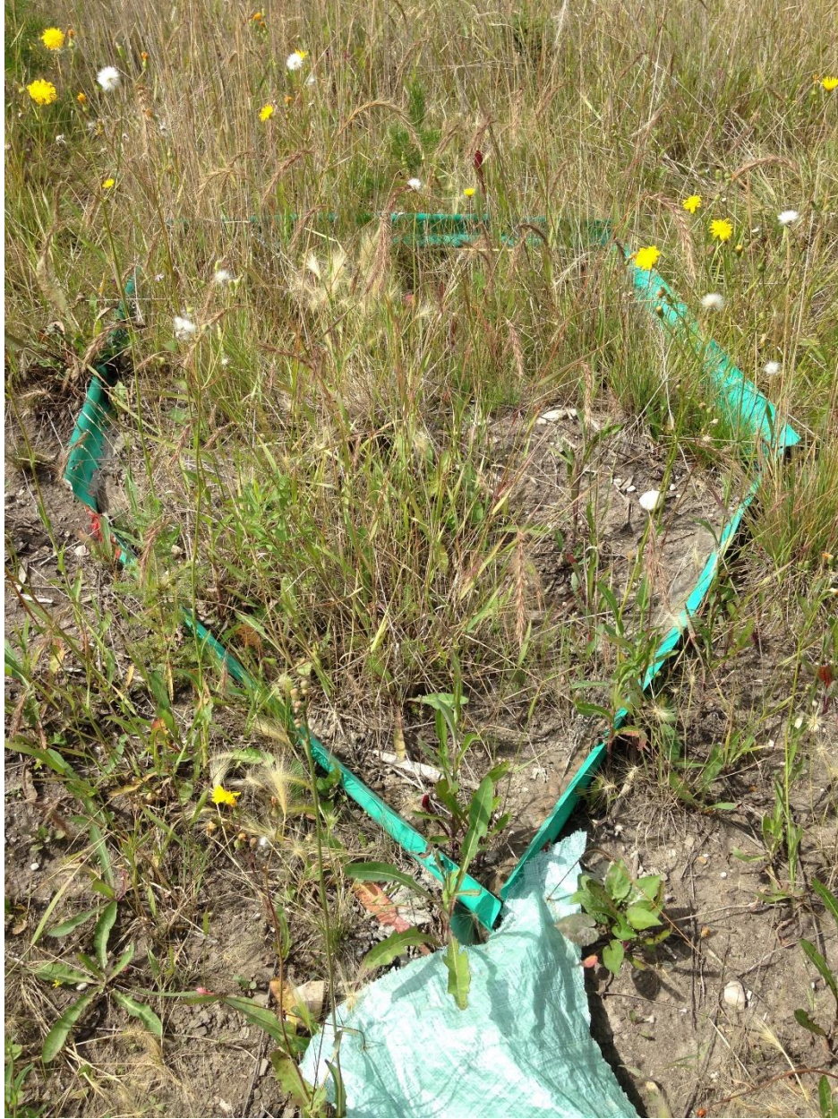
Figure 3-2. An enclosed runoff collector, located on the west slope, used to collect DOC samples in 2015, and estimate runoff depth in 2015 and 2016. Vegetation cover is limited, and vegetation height in this photo does not exceed 0.5 m.
