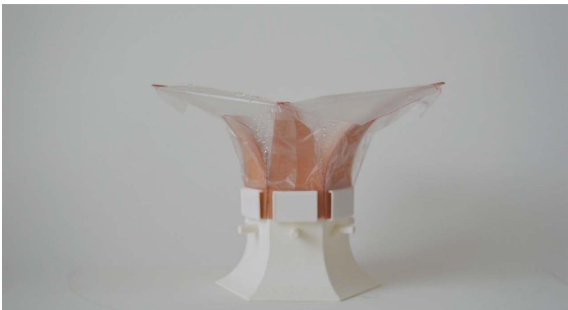
FIG. 32 FINAL PROTOTYPE MOTION The image shows the final assembly of the hygroscopic mechanism in its open state.
