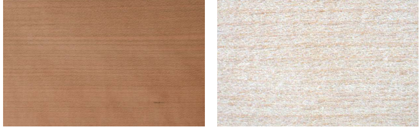
FIG. 16 (BELOW) EUROPEAN BEECH BILAYER: GRAIN ORIENTATION
