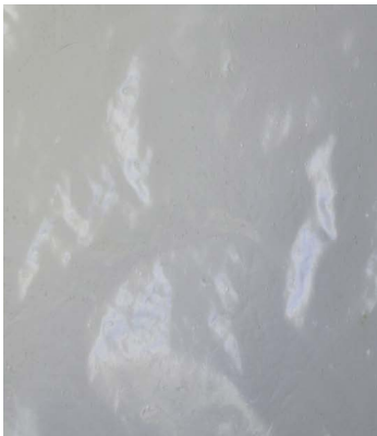
FIG. 19 STARCH BASED BIOPLASTIC TEST B The image shows the results of the second test of producing starch based bioplastics. This test incorporated gelatin to the original mix to strengthen and improve elasticity.
