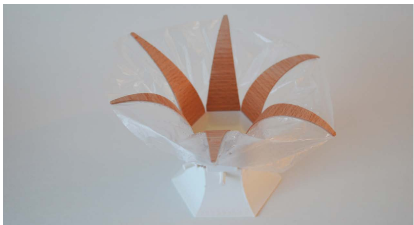
FIG. 36 FINAL PROTOTYPE MOTION The image shows the final assembly of the hygroscopic mechanism in its open state.
