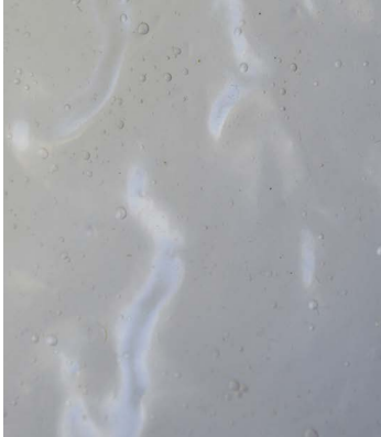
FIG. 18 STARCH BASED BIOPLASTIC TEST A The image shows the results of the first test of producing starch based bioplastics. This test used a combination of water, corn starch, glycerin and vinegar to produce a translucent flexible plastic.
