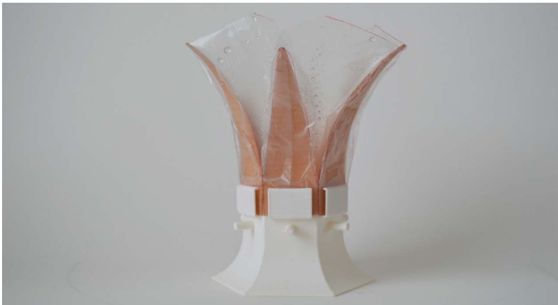
FIG. 31 FINAL PROTOTYPE MOTION The image shows the final assembly of the hygroscopic mechanism in its partially open state.
