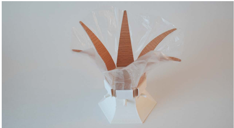
FIG. 35 FINAL PROTOTYPE MOTION The image shows the final assembly of the hygroscopic mechanism in its partially open state.
