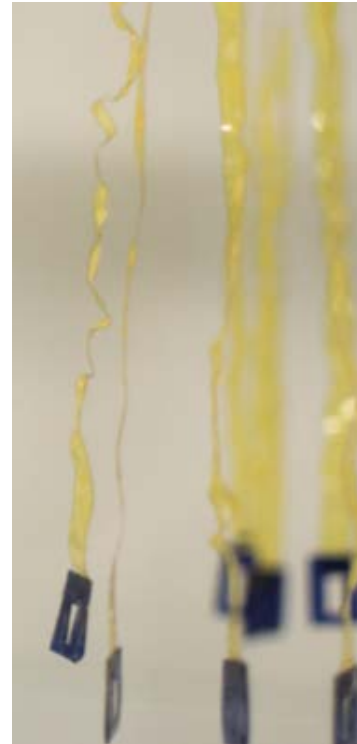
FIG. 24 BIOLOGICAL HYGROMORPHS Application of bacterial spores onto passive plastic strips result in a contraction of the strip when in the presence of moisture. Photo retrieved from: Ramirez-Figueroa, C., L. Hernan, A. Gnyet, and M. Dade-Robertson. "Bacterial Hygromorphs: Experiments into the integration of soft technologies into building skins." 2016.
