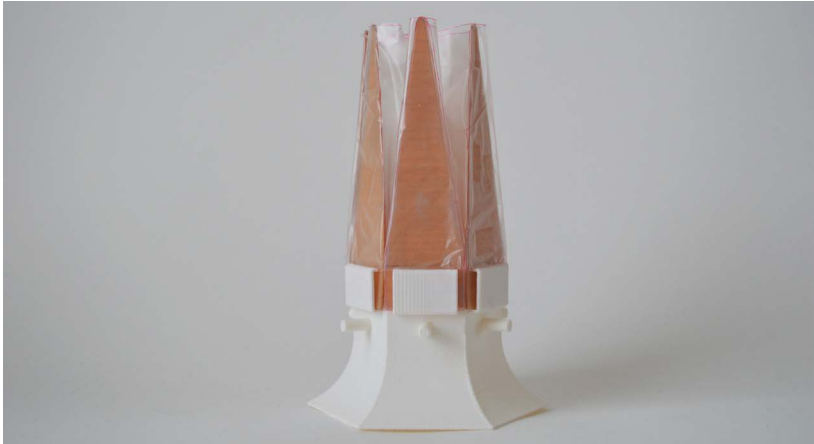
FIG. 29 (FACING PAGE) FINAL PROTOTYPE MOTION The image shows the final assembly of the hygroscopic mechanism in a still visualization of the completed motion from closed to entirely open.
