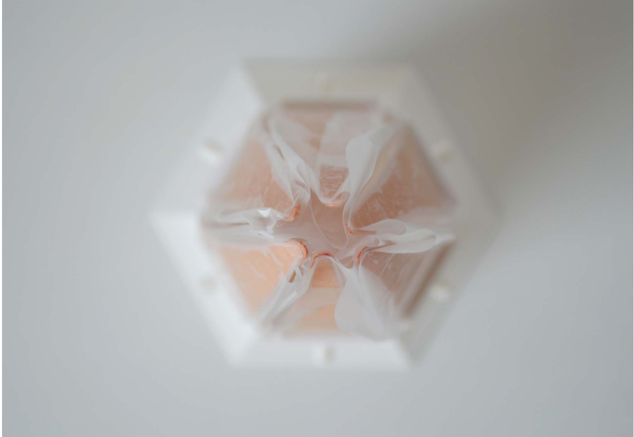
FIG. 25 (ABOVE) FINAL PROTOTYPE The image shows the final assembly of the hygroscopic prototype from above, demonstrating the clustering of the mechanisms composites to a point.
