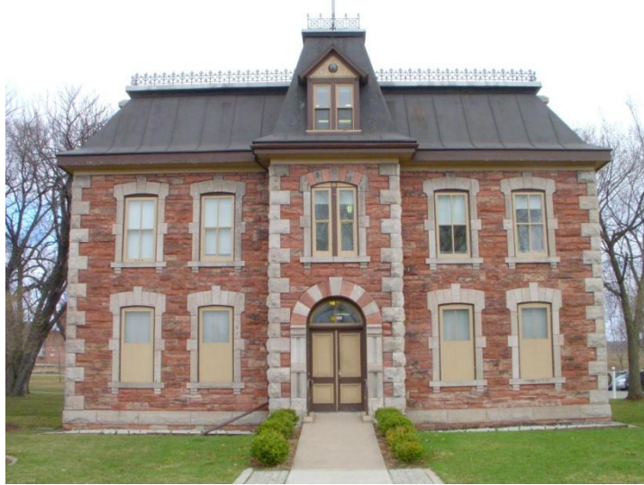
Figure 8 - Example of Second Empire Style Building with Central Pavilion and Mansard Roof
