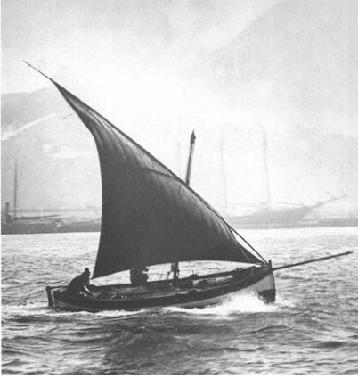
Figure 1.03. A lateen rigged felucca, mimicking the style of ancient Greek boats.
