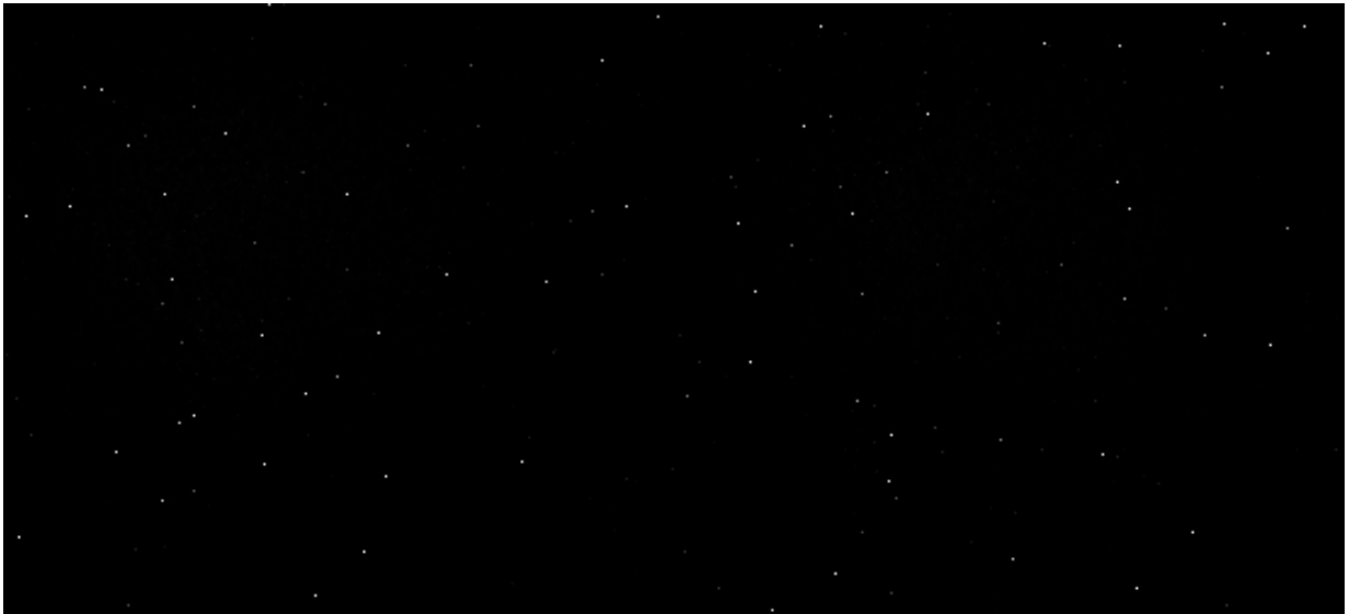
Figure 2.38: A picture taken with the photon camera not capped while single photons are being imaged at an intensifier gain of 21 and an EM gain of 58 for 100,000 On-CCD Accumulations with 500 frames
