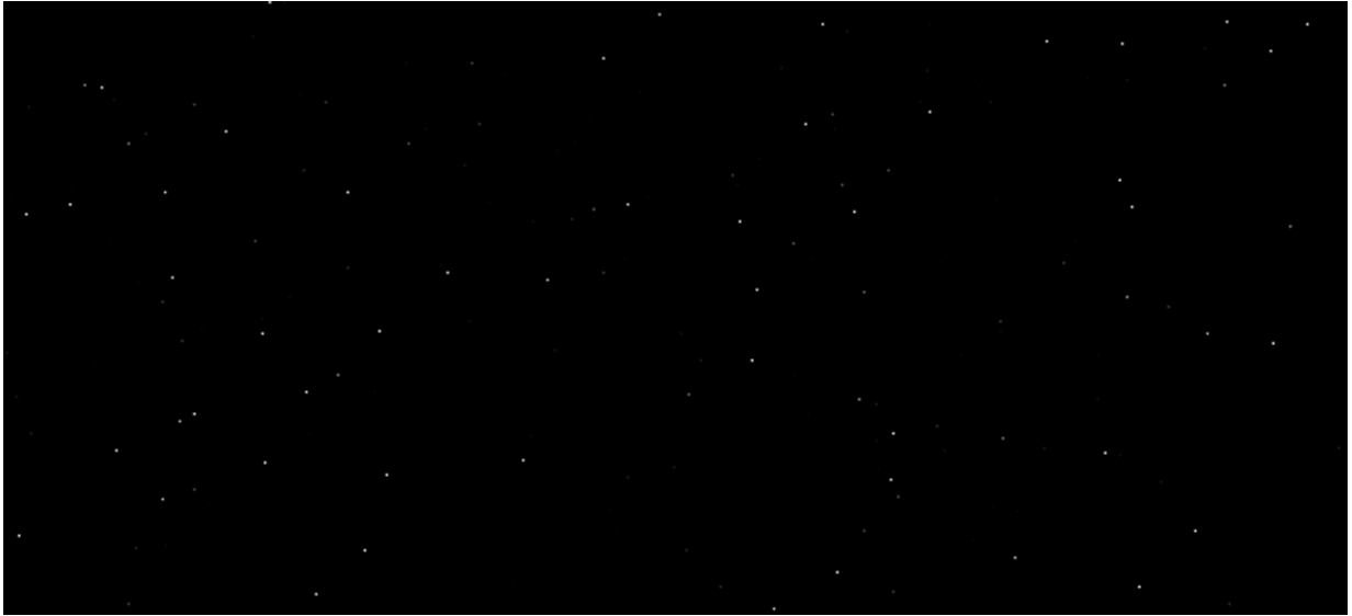
Figure 2.37: A picture taken with the photon camera capped at an intensifier gain of 21 and an EM gain of 58 for 100,000 On-CCD Accumulations with 500 frames
