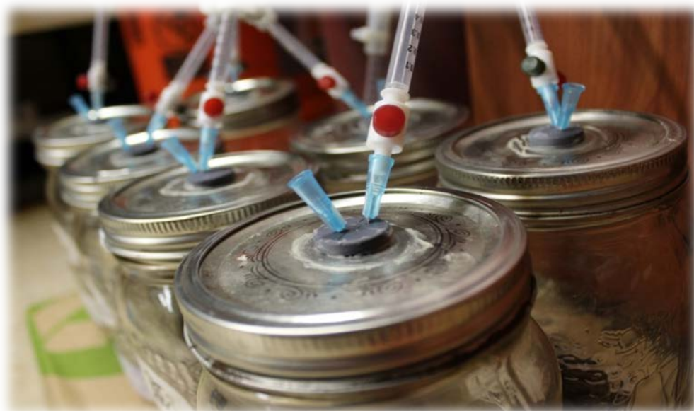
Figure 2.5 UHP-He flushing the jars in the DNIT process through a valve regulator attached to one needle; the second needle was used to release the oxygen out of the system.
