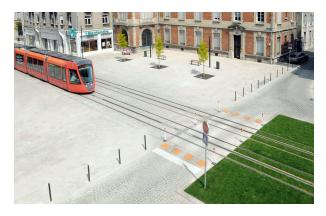
**FIGURE 4-3** Catenaryless LRT systems eliminate unsightly overhead wires and poles, and can easily transition between varied surfaces.
