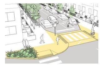
**FIGURE 4-5** Curb bump-outs and raised crosswalks increase pedestrian safety at crossings, while also providing space for bioswales at the end of parking zones.
