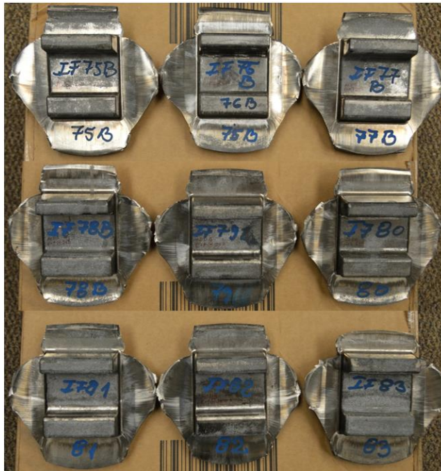
Fig 64: Photographs of extruded AZ31B closed-die forged at 250°C.
