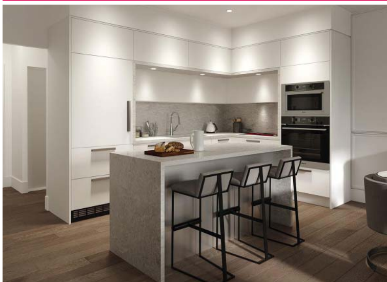
Bar-height surfaces, lack of knee space, unreachable upper cabinets
