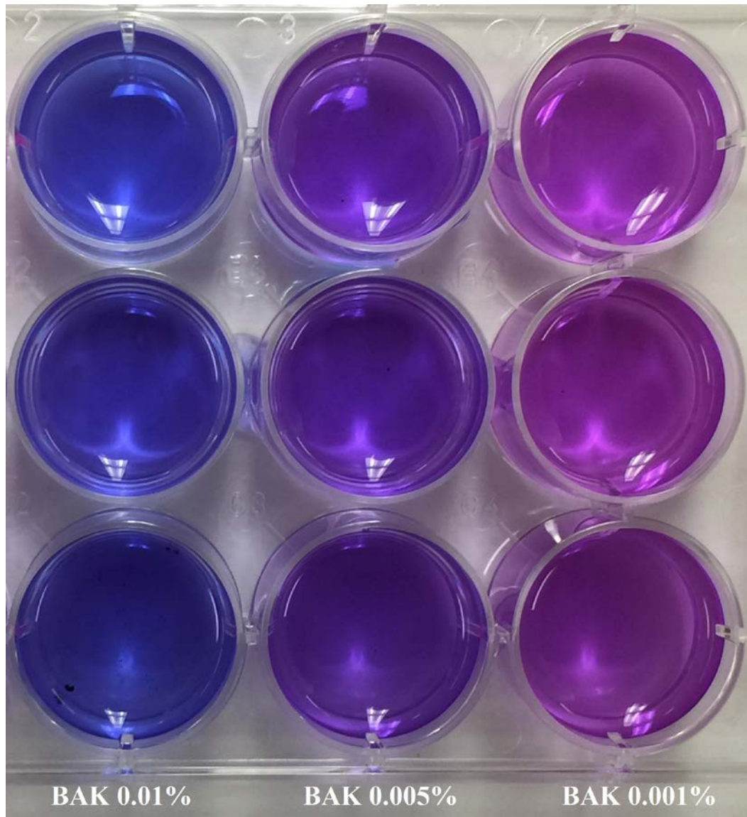
Figure III-2 End-point appearance of the alamarBlue assay for control and BAK-treated lenses. AlamarBlue (blue) is reduced to fluorescent alamarBlue (red) proportional to cellular metabolic activity.
