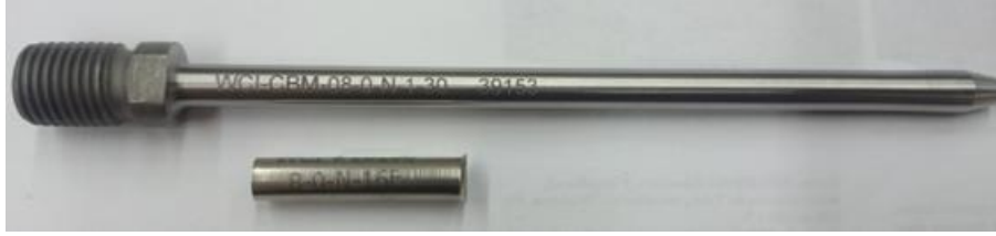
Figure 21. Mandrel and split sleeve
