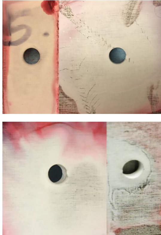
Figure 45. Dye penetrated DCE sample, from left to right: 2,4,5,6 % DCE
