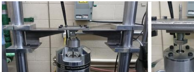
Figure 27. Designed structure mounted on MTS, (left), detailed view of the work piece and mounted split sleeve (right)
