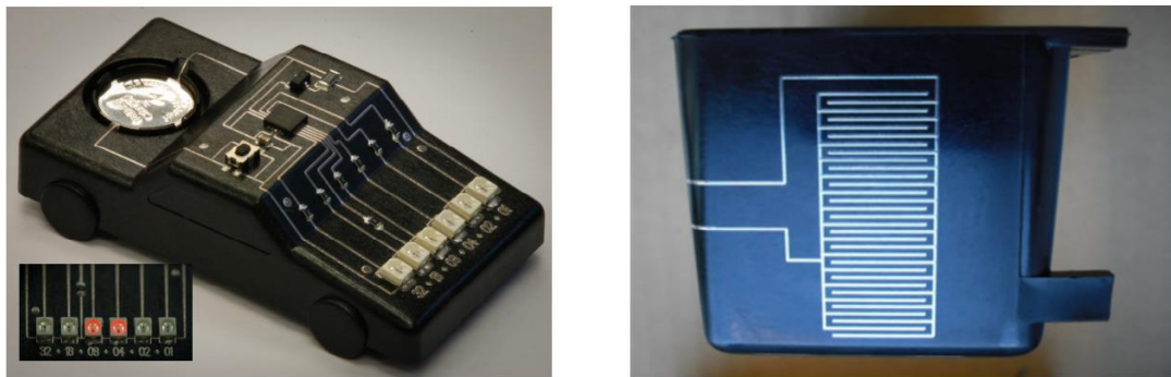
Figure 2.3: Demonstrations of Optomec M 3 D Aerosol Jet Printer: (Left) Digital thermometer on PA10 thermoplastic, (Right) Detail of capacitive sensor structure
