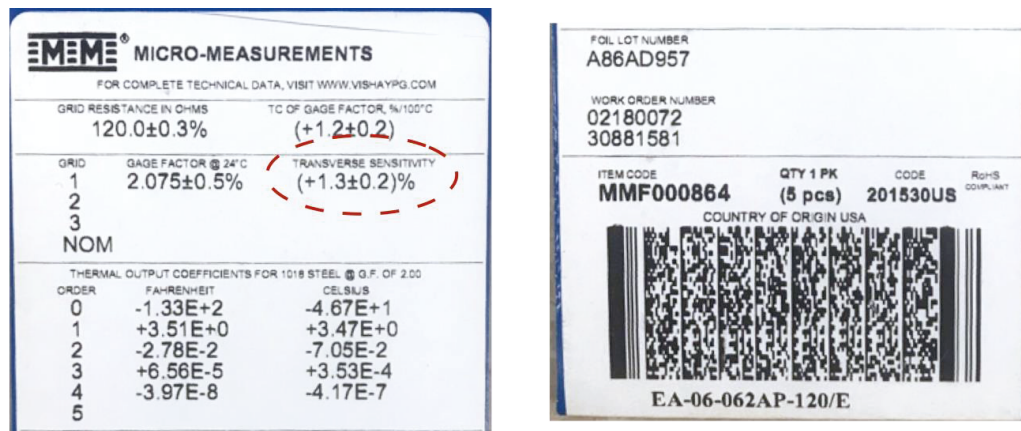
Figure 3.11: EA-06-062AP-120/E strain gauge from micro-measurements highlighting transverse sensitivity value
