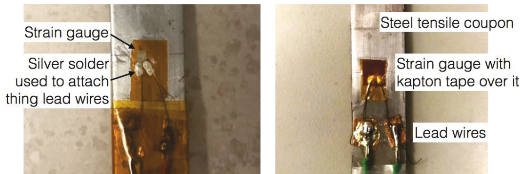
Figure 4.8: (Left) Uncovered printed strain gauge showing strain gauge and silver solder on tensile coupon. (Right) Kapton tape placed over printed strain gauge for protection
