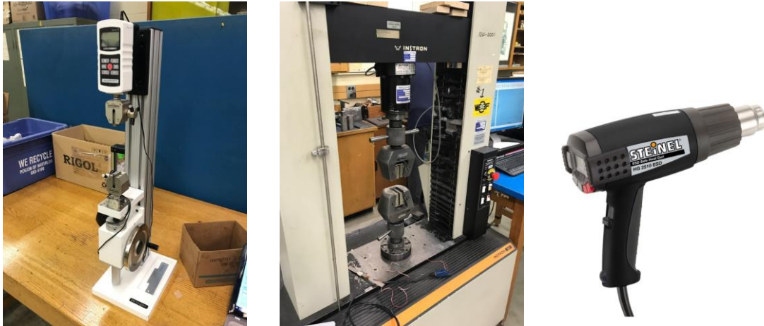
Figure 4.9: (Left) Manual hand-operated tensile tester, (middle) electric programmable tensile tester and (right) heat gun
