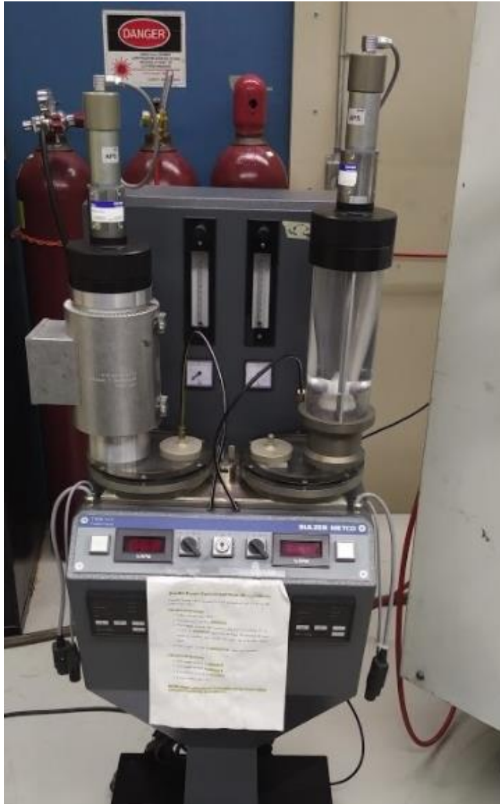
Figure 7.2: Powder delivery apparatus
