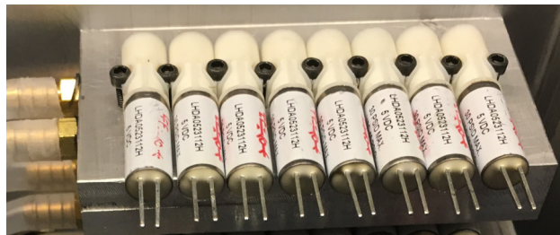
(c) A picture of an aluminum module mounted within a system. The input tubing is now much larger (1/8" ID tygon tubing) and more easily connected.
