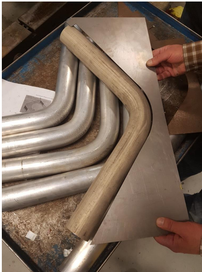
Figure 6.4-22: Checking bend angle against the bend gauge
