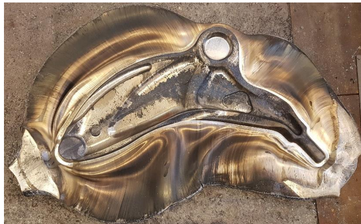
Figure 6.4-13: Forging trial result for ZK60 forged at 450 °C.
