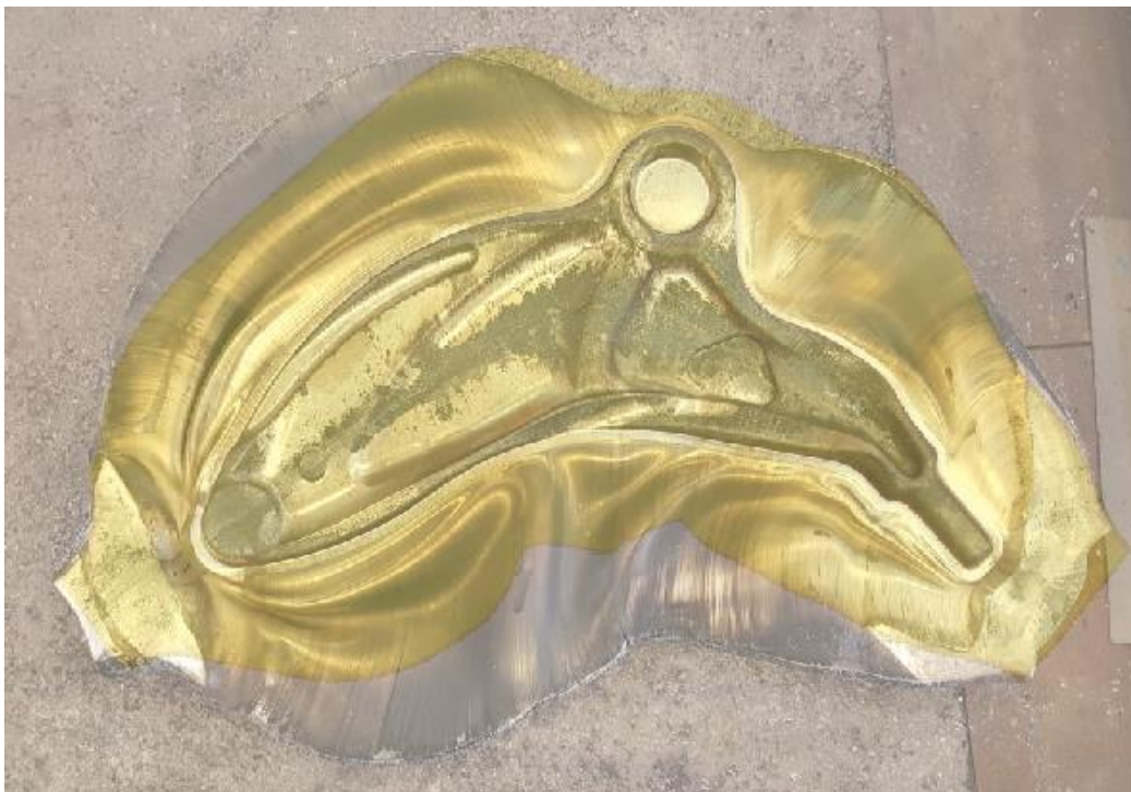
Figure 6.4-16: ZK60 geometric comparison with simulation. Yellow is the model-predicted final forged geometry overlaid on the actual forging.
