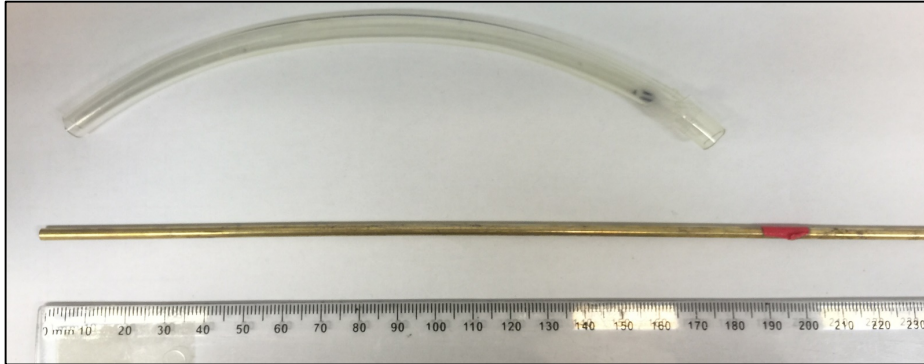
Fig. S1. The medical-grade PU tubing (7.95 mm in cross-sectional diameter, 0.78 mm in wall thickness, 85A shore hardness) and copper rod used for implantation procedure. Units in mm.
