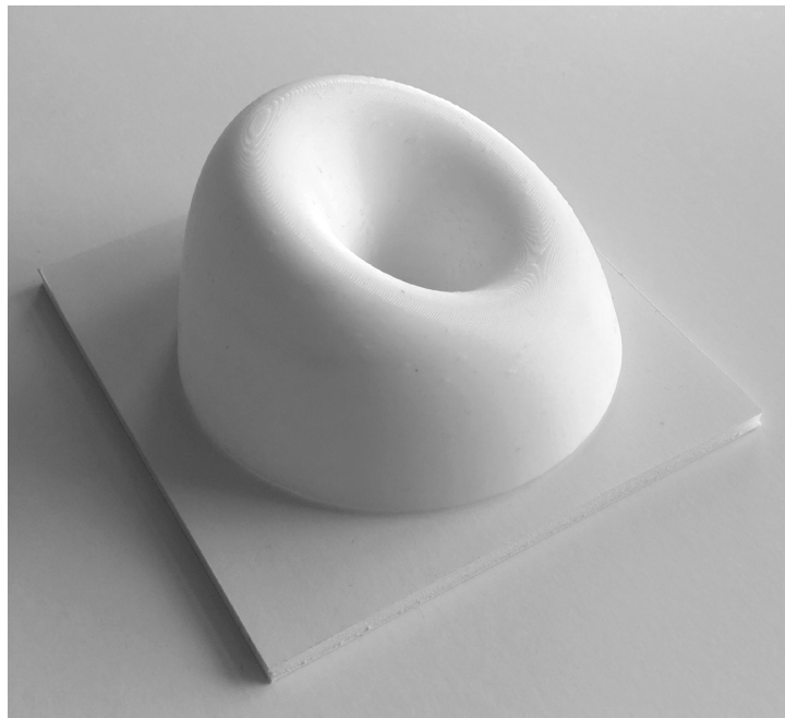
Figure 5.10 - Half 3D printed test model showing potential buildup of interior walls
