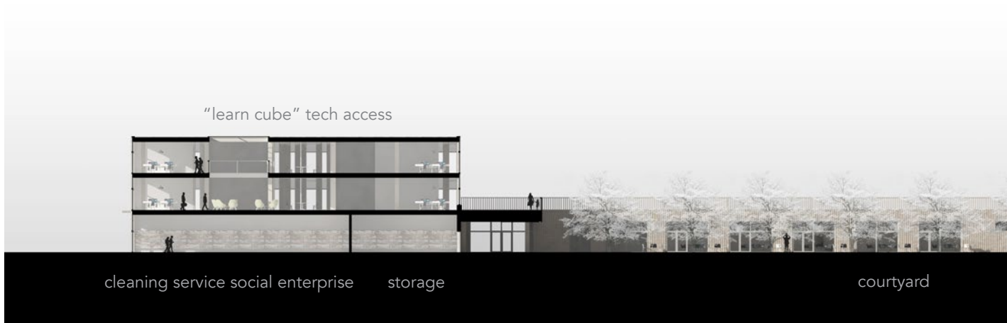
Fig. 4.36 Section BB . Image by Xiao Wen Xu. The learning programs are stacked on top of the job enterprises in the Learn Cube. Moving north, underneath the ramped track, is a covered walkway. The dogwood trees in the courtyard serve as an outdoor screen with their delicate low-lying foliage.
