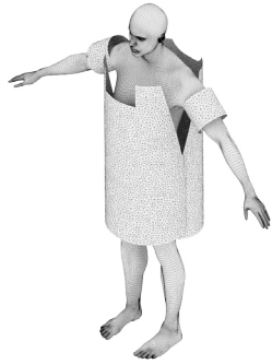
Figure 017 Mesh wrapped to corresponding cylinders
