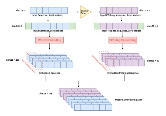
Figure 5.2: Word and Pos-tag encoding layer
