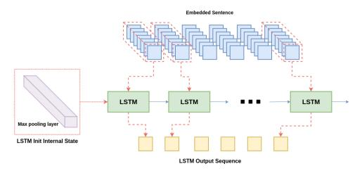
Figure 5.5: LSTM decoder layers
