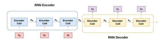
Figure 2.3: RNN Encoder-decoder Architecture
