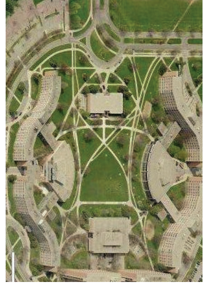
Fig. 4.11 Soft Scaffold: Michigan State University. Desire paths from trails formed by walking are paved over as hardscape paths.
