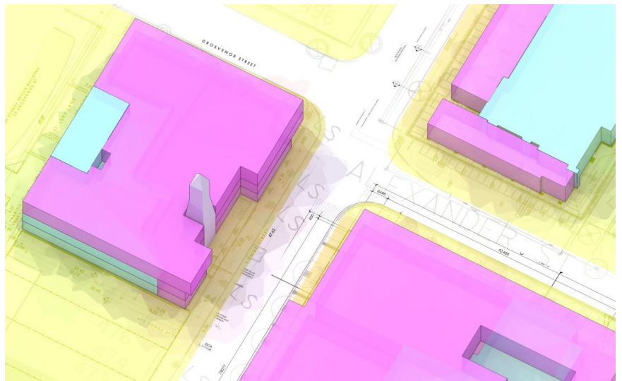
Fig. 2.34 Rendering showing existing curblines in yellow with approved building cores in blue and commercial spaces as pink.
