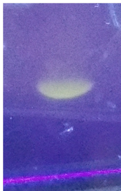
Figure 2.2: NBD-labelled CAMP factor Mutant on SDS-PAGE. Ultraviolet trans-illuminated SDS-PAGE gel of F138CNBD. Cysteine mutant F138 was labelled with IANBD with high labelling efficiency in TCEP-containing sodium phosphate buffer (100 mM sodium phosphate buffer with 1 mM Tris (2-carboxyethyl) phosphine (TCEP), pH 7.3) and purified via gel filtration.
