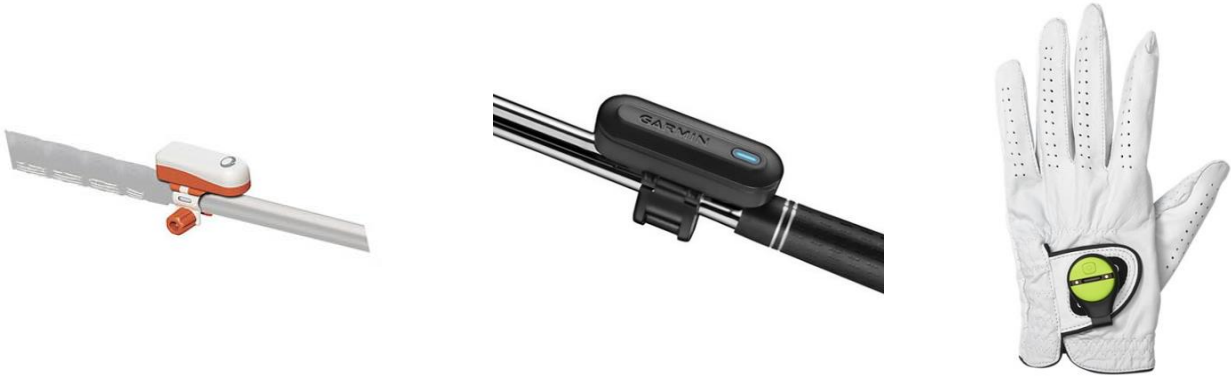
Figure C.1 - The 3 IMU devices tested: SkyPro (left), Garmin TruSwing (middle), and the Zepp Golf 2 (right).
