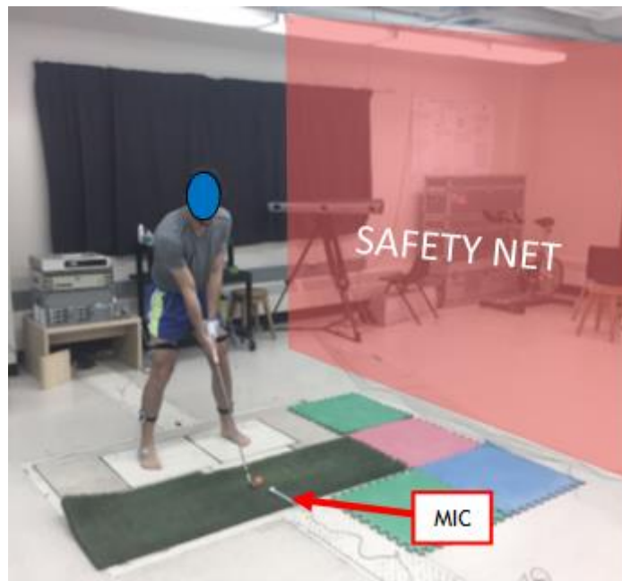
Figure 3.2 – Setup showing the turf overtop FP1 and FP3, surrounding mats, foam golf ball, and microphone. Golf netting used as a safety barrier to the equipment and study investigator (black mesh highlight in red).
