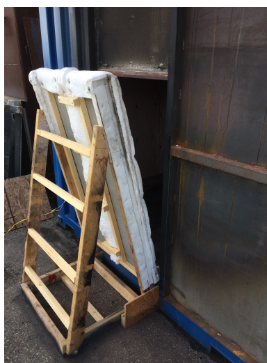
Figure 6.1: Obstruction angled at 15 degrees in front of the single opening; taken from [27].
