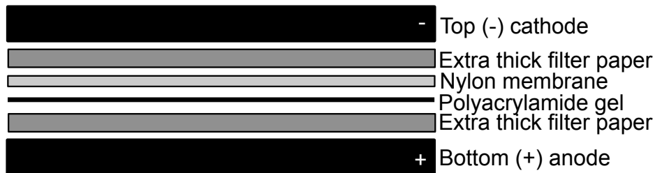
Figure A.5. The order of assembly for a dsRNA immunoblot transfer. From the bottom anode up, the stack should include a layer of extra thick filter paper, a nylon membrane, the polyacrylamide gel, and another layer of extra thick filter paper. The membrane and filter paper should be presoaked in transfer buffer (0.5X TBE).
