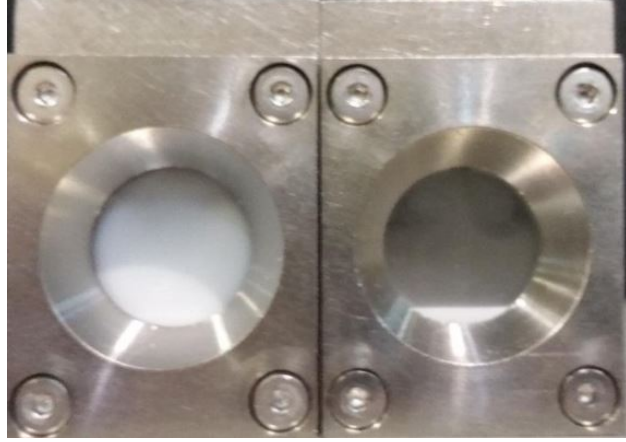
Figure 2.20: Photo of the sample holders for the polystyrene sphere solution about 3 weeks after the measurements. The 4 mm thick holder is on the left and is clearly turbid, while the 1 mm thick holder is on the right showing that the spheres have settled out. Figure taken from Ref. [13].
