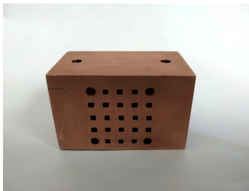
Figure 7.16: The photo of the copper collimator with 5 \times 5 openings.
