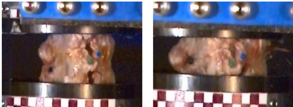
Figure 108: Specimen #28 in centric compression case (left: at the start of the experiment, right: during compression) [Carter, 2002]
