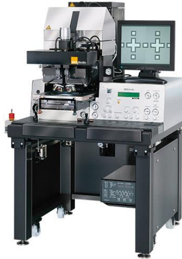
Figure 2.1 MA/BA6 Mask and Bond Aligner (Courtesy to SUSS MicroTec).
