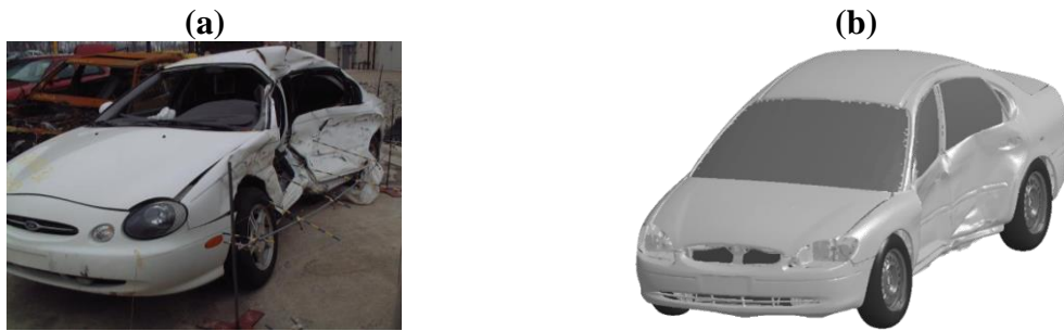
Figure 3.9: Deformation pattern (a) of the physical vehicle (CIREN 2018), (b) predicted by the computational model.
