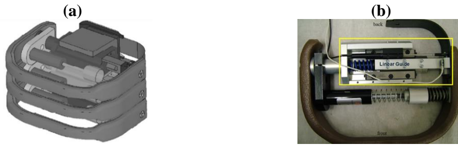
Figure 2.8: (a) Computational model of the side impact ES-2re ATD thorax, (b) ES-2re rib potentiometer (Stricklin 2009).
