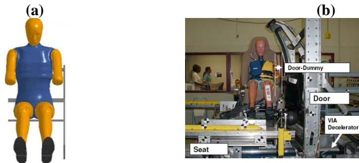
Figure 2.7: (a) Computational model of the ES-2re ATD (DYNAmore 2015) integrated with a rigid-wall sled model, (b) physical component test utilizing the ES-2re ATD (Aekbote 2007).
