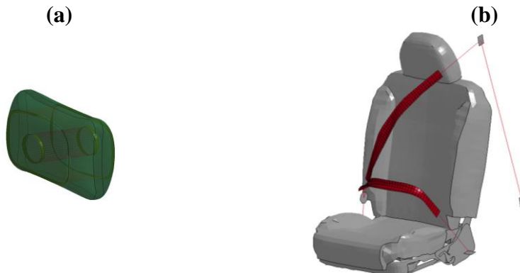
Figure 6.1: Restraint models: (a) inflated tSAB, (b) seat with a three-point seatbelt.
