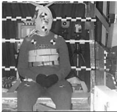
Figure 2.4: Instrumented PMHS prepared for a rigid-wall sled test (adapted from Pintar 2007).
