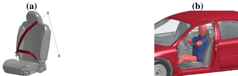
Figure 2.26: Numerical models of the: (a) seat (gray) and a three-point seatbelt (red), (b) UW-HBM integrated with the vehicle. Side door removed for clarity.
