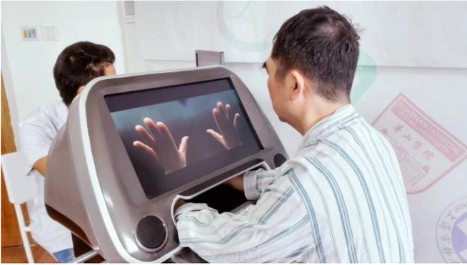
Fig. 1. The camera-based mirror visual feedback setup.
