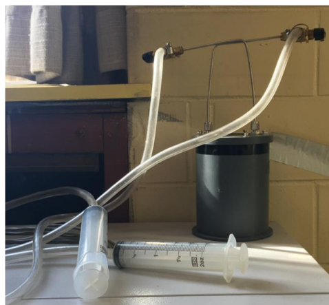
Figure 61: (A) inside and (B) outside of gas evolution apparatus
