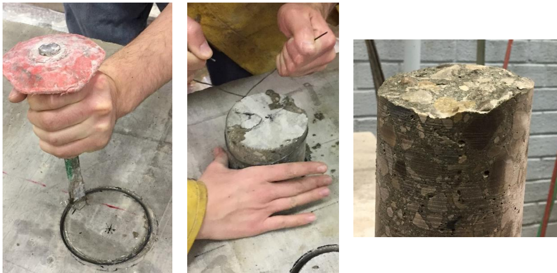
Figure 3.4 Core Removal Process
