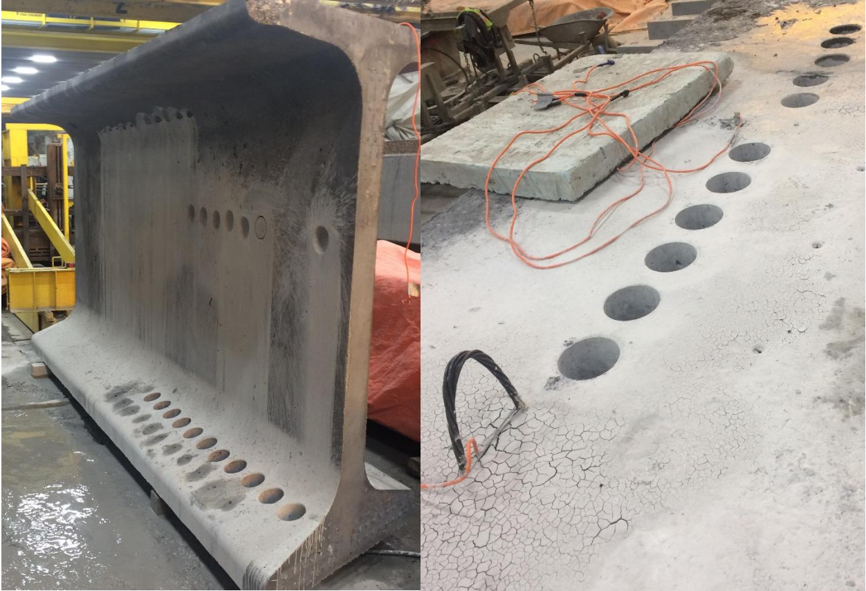
Figure 3.17 Day 3 Core locations in G3 Girder
