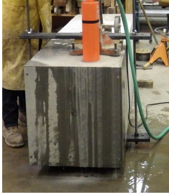
Figure 3.3 Coring drill clamping assembly for UW lab beams
