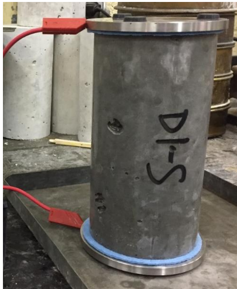
Figure 3.27 Bulk Resistivity Measurement
