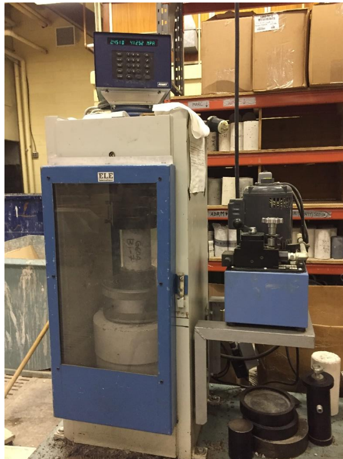
Figure 3.28 Hydraulic Compressive Testing Machine in the UW Lab
