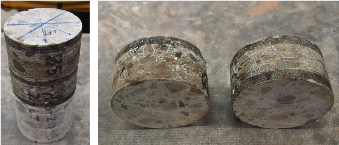
Figure 3.26 Rapid Chloride Permeability Test Samples from B2 Beams
