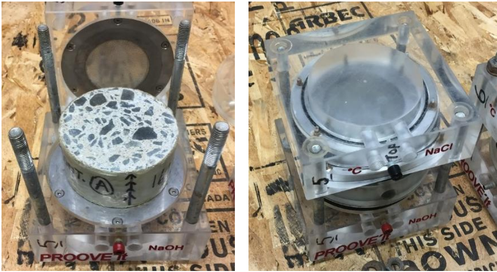
Figure 3.25 Rapid Chloride Permeability Test Set-up
