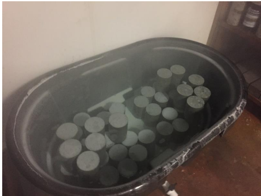
Figure 3.24 Sealed and Soaked Conditioning of Cores
