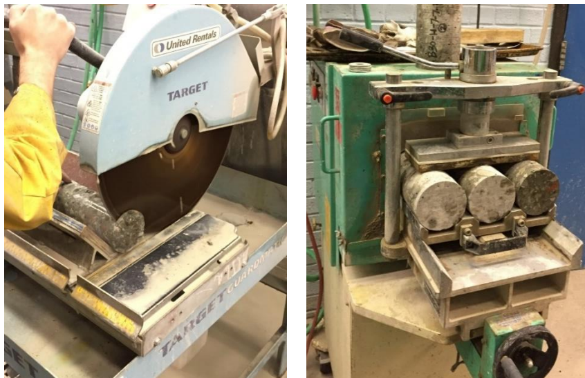
Figure 3.23 Cutting and end-grinding of cores
