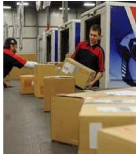
Figure 1.1: Randomly-oriented packages moving on a conveyor in a non-singulated manner (courtesy of Purolator Inc.)
