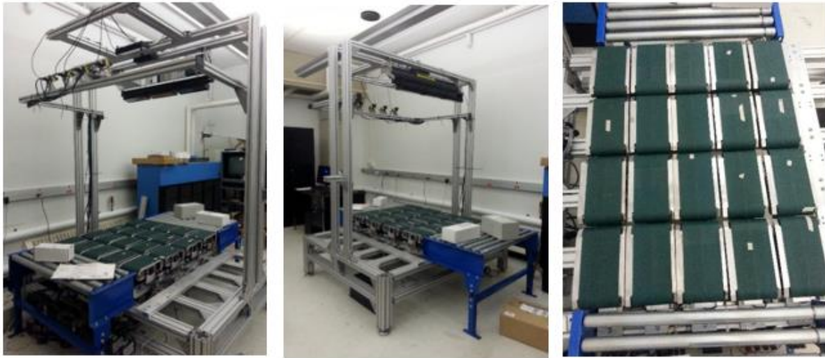
Figure 2.7: Final prototype of IMWS Array system
