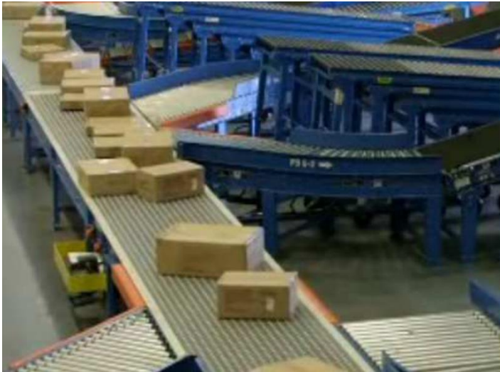
Figure 1.1: Randomly-oriented packages moving on a conveyor in a non-singulated manner (courtesy of Purolator Inc.)
